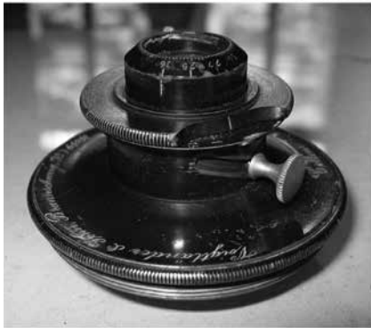
Illustration 44 – The Voigtlander lens on the first prototype of the Cinématographe. Photographs by Jean-Marc Lamotte, Institut Lumière.
