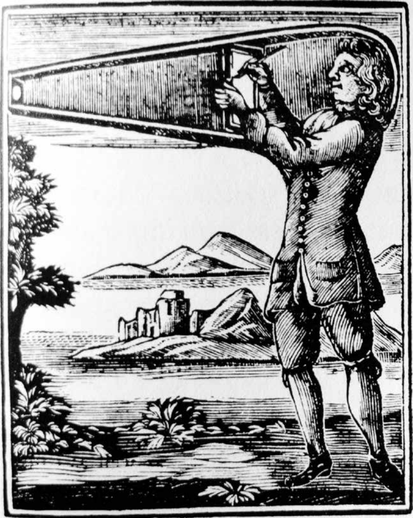
Illustration 11 – Robert Hooke's portable Camera obscura (1694). From John H. Hammond, The Camera Obscura: A Chronicle .
