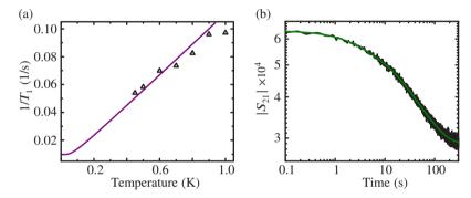
**Figure 6.4:** (a) Temperature dependence of the spin-lattice relaxation time. The purple line is a fit assuming a direct relaxation process. (b)  $|S_{21}|$  decay curve after a saturation pulse, plotted in double-logarithmic scale. The decay strongly deviates from a simple exponential decay curve. The green line is a fit employing a sum of three exponential decays. After  $100 \, \text{s}$ ,  $\gtrsim 90\%$  of the spins are relaxed back to equilibrium.
