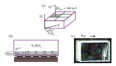
**Figure 5.15:** (a) Sketch of the implantation process. A focused  $Er^{3+}$  ion beam irradiates several areas of an undoped  $Y_2SiO_5$  crystal. (b) Schematics of the coupling geometry. (c) Picture of the implanted YSO crystal on top of a superconducting chip with an array of nine LE resonators. Each implanted area fits to the size of one LE resonator.
