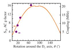
**Figure 5.19:** Collective coupling strength vs. rotation angle  $\theta$ . The solid line shows the simulated AC g-factor for the  $S_{2b}$  transition. The size of the points covers the approximate uncertainty of the data.
