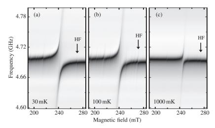
**Figure 5.9:** Avoided level crossing at different temperatures. Remarkably, the hyperfine transitions are more pronounced at 100 mK, and the system is still strongly coupled at 1 K,.
