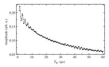
**Figure 6.11:** Stimulated echo decay. The beating between the two hyperfine frequencies is clearly visible. The data can be fit with a double exponential decay with decay times of 2 and  $23.9 \,\mu s$ .
