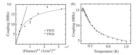
**Figure 5.17:** (a) Collective coupling vs. the square root of the fluence. The dashed straight line shows the expectation for a 100% effective implantation. The gray line is a fit to an empirical theory, see text for details. (b) Temperature dependence of the collective coupling strength of sample YSO4 area #3. The temperature dependence follows the expectation for a paramagnetic crystal (gray line).
