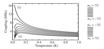
**Figure 5.11:** Simulated temperature dependencies for the coupling strengths of the hyperfine transitions of <sup>167</sup>Er.
