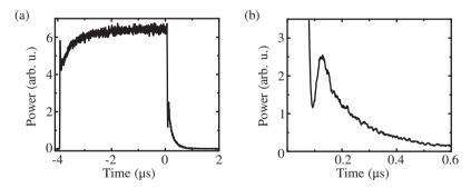
**Figure 6.7:** (a) Transmitted resonant microwave power vs. time. The beginning and end of the pulse shows a characteristic oscillation. (b) Zoom onto the oscillation at the end of the pulse.
