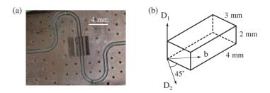
Figure 6.1: (a) Crystal on copper CPW resonator. (b) Orientation of the crystal.
