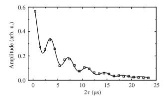
**Figure 6.10:** The exponential echo decay is modulated by prominent oscillations. The solid line presents a fit to the data with a  $T_2$  time of 5.6  $\mu$ s.
