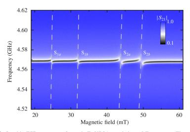
Figure 5.2: On-chip ESR spectrum of sample Er:YSO1 coupled to a LE resonator. The orientation of the crystal's b-axis with respect to the DC magnetic field is  $\theta = 81.3^{\circ}$ .
