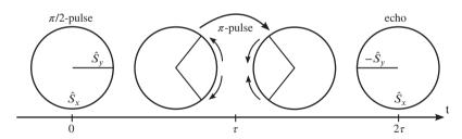
**Figure 2.4:** From left to right, spin dynamics of the two pulse sequence in the equatorial plane of the Bloch sphere. After the initial  $\pi/2$ -pulse, the spins defocus. At  $t = \tau$ , the  $\pi$ -pulse flips the phase of the y-component leading to a rephasing and an echo at  $t = 2\tau$ .
