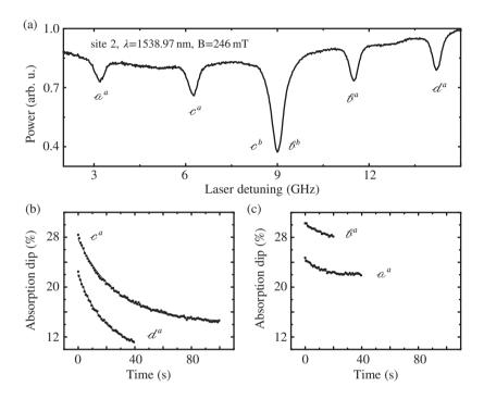
**Figure 7.5:** (a) Optical transmission at 246 mT. (b) Time evolution of the absorption dips of transitions  $e^a$  and  $d^a$  after a strong microwave pulse on the  $|g\downarrow\rangle$  to  $|g\uparrow\rangle$  transition of site 2a (site  $2^a$ ). (c) Corresponding time evolution of the absorption dips of the  $e^a$  and  $e^a$  transitions.
