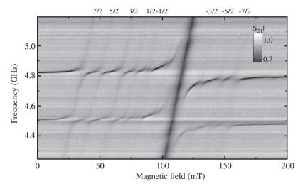
**Figure 5.13:** Avoided level crossings between the two LE resonators and the Nd spin ensemble. The coupling to the hyperfine transition is clearly visible.
