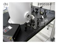
**Figure 4.5:** Second small optical table at the cryostat. (a) The laser beam is coupled out of the fiber, linear polarized, widened to approximately 1 cm diameter and finally focused into the fridge. In the background, the Thorlabs PDA10CS photodetector is seen. (b) Optical output of the cryostat. The beam is focused on the AOM switching it between two photo detector.
