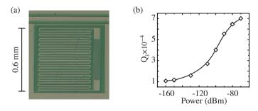
**Figure 4.4:** (a) Optical micrograph of a LE resonator. (b) Power dependence of the internal quality factor. The solid line is a guide to the eye.
