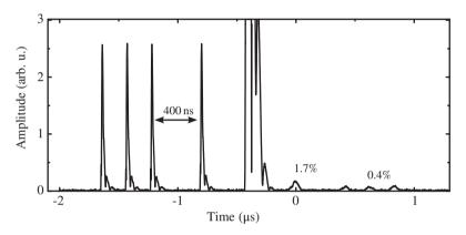
**Figure 6.15:** Storage and retrieval of four irregularly spaced MW pulses. The strong  $\pi$ -pulse in the middle extends far beyond the graph's vertical axis. The presented data is the result of 18 averages with a repetition rate of 10 mHz.
