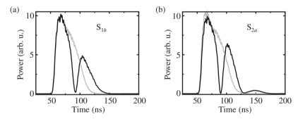
**Figure 6.8:** Response to a 20 ns MW pulse. The grey line shows an off resonant pulse for comparison. (a)  $S_{1b}$  transition (143.0 mT). (b)  $S_{2a}$  transition (245.8 mT).
