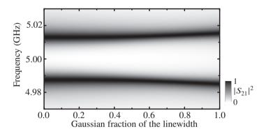
**Figure 3.4:** Power spectrum as a function of probe frequency for different inhomogeneous spin line shapes from purely Lorentzian (left) to purely Gaussian (right).
