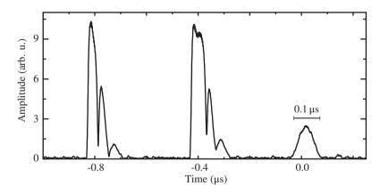
**Figure 6.9:** Spin echo sequence with a pulse separation of  $\tau = 400$  ns. Each pulse is accompanied by vacuum Rabi oscillations. The  $\pi/2$ -pulse has a width of 20 s, but the echo appears as a 100 ns wide pulse of approximately Gaussian shape.
