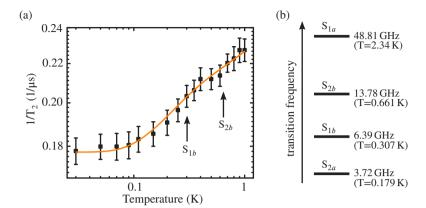
**Figure 6.13:** (a)  $1/T_2$  vs. temperature. Note the logarithmic scale. Between 30 mK and 1 K, the  $T_2$  time decreases from approximately 5.6  $\mu$ s to 4.4  $\mu$ s. The solid line is a fit to theory considering decoherence induced by thermal fluctuations from the surrounding sub-ensembles. (b) Transition frequencies and effective temperatures at 246 mT of all sub-ensembles.
