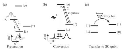
**Figure 3.5:** Schematics of an optical-to-microwave conversion protocol.
