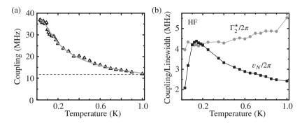
**Figure 5.10:** (a) Temperature dependence of the collective coupling strength of the  $S_{2a}$  transition coupled to the LE resonator. The solid line is a fit to the theory and the dashed line indicates the level of the inhomogeneous spin linewidth. (b) Temperature dependence of coupling strength and linewidth of the hyperfine line "HF". The coupling is strongest around 140 mK and approaching the strong coupling regime.
