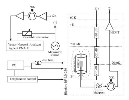
Figure 4.3: Setup for continuous wave microwave on-chip spectroscopy. The sample is placed inside a solenoid coil and cooled down to  $20 \, \text{mK}$ . Typical probing powers at the sample range from  $-120 \, \text{dBm}$  to  $-140 \, \text{dBm}$ . Cold attenuators, a cryogenic circulator and HEMT ensure a good signal-to-noise ratio down to the single photon regime.
