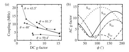
**Figure 5.5:** Anisotropic coupling. (a) Coupling vs. DC g-factor. For almost all samples, the coupling scales inversely to the DC g-factor. (b) Simulated angular dependence of the AC g-factor for  $\theta=44^\circ$ . The grey line denotes the mean orientation. The coupling measured with on-chip ESR represents an average value with respect to the AC g-factor anisotropy due to the inhomogeneous AC field of the LE resonator.
