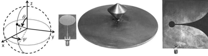
Fig. 6.9.: The spherical coordinate system and three antennas used during measurements. From left to right: planar monopole, monocone- and Vivaldi-antenna.
