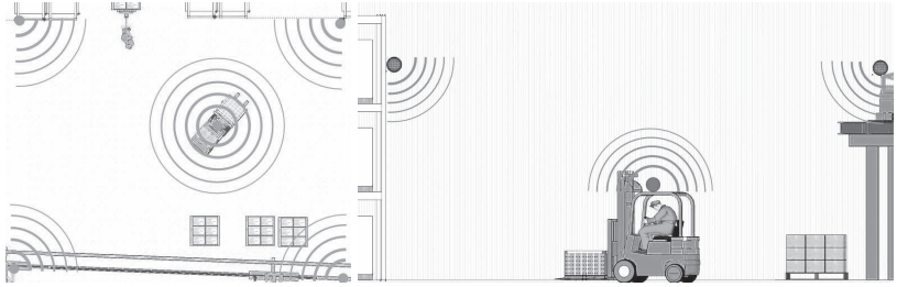
Fig. 6.8.: Top and side view on an example indoor scenario, showing the placement of the APs and an exemplary position of the MU. The favored antenna characteristics in horizontal and elevation direction are marked with circular lines.
