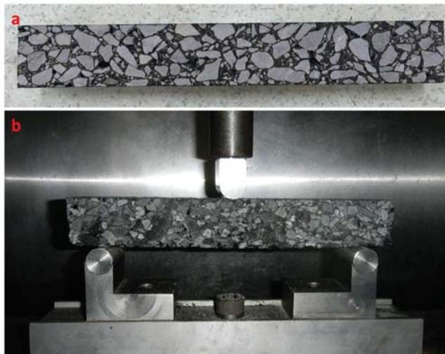
Figure 2. Specimen and setup used for three-point bending test: (a) prismatic beam; (b) test setup.
