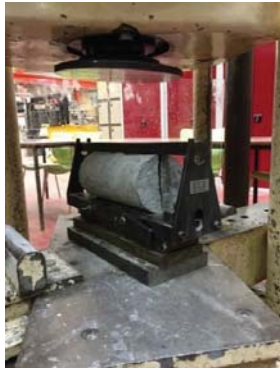
Figure 9. Splitting tensile test.
