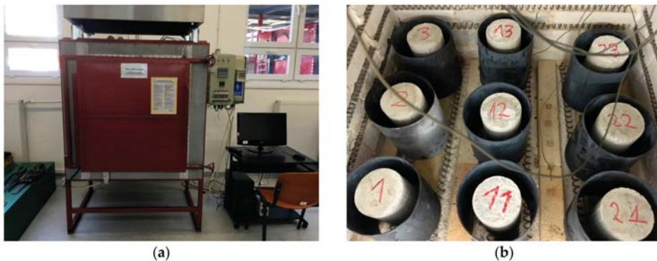
Figure 1. (a) Furnace for samples annealing, (b) Samples in the furnace chamber secured by steel covers.
