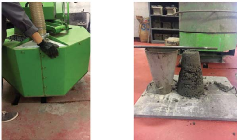
Figure 5. Concrete mixer (left); concrete slump test (right).
