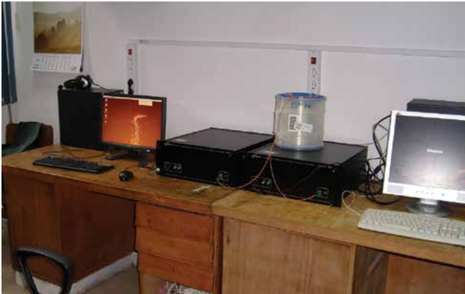
Fig. 12. Communication line setup used in the QUANTGRID D11-044 project (Inst. for Laser and Plasma Phys. – Bucharest), with its two dedicated computers (Bob – receiver and Alice – sender). The quantum channel (23.845 km) optical fiber spool is on top of the Bob station. The classical channel linking the computers is local LAN Ethernet.
