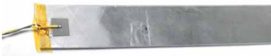
Fig. 1. A PZT patch bonded to an aluminum beam for damage detection.
