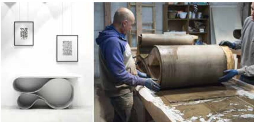
Figure 4. The Whorl Console made with the concrete cloth technology [29].
