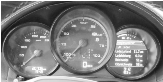
Figure 25: On the right side of the dashboard, the value of different services such as SOC, range capability, battery capacity, range in the city and charging time are displayed.
