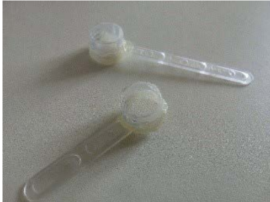
Fig. P22.3. Milliliter "dip net" to measure 2ml of fly larvae. (photo: F. Chardonnet).
