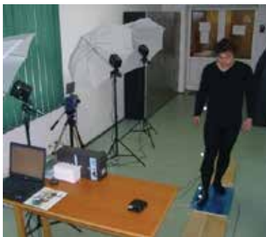
Fig. 14. Acquiring and measuring system, Biopac type, for the foot and lower leg linear accelerations
