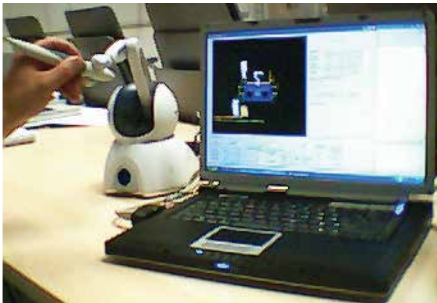
Fig. 6. Off-line programming of the telerobot using a haptic device
