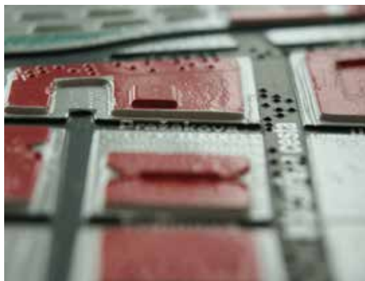
Fig. 1. Relief structure (layers) of the tactile map.
