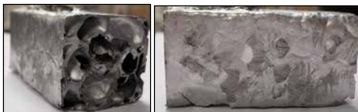
Fig. 9. Shaped MGI part with dense skin
