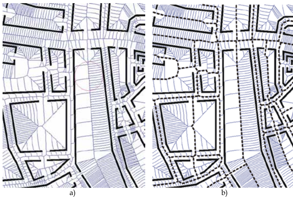
Fig. 4. Construction of the GVD: a) ordinary Voronoi diagram (light lines), b) GVD (dotted lines)
