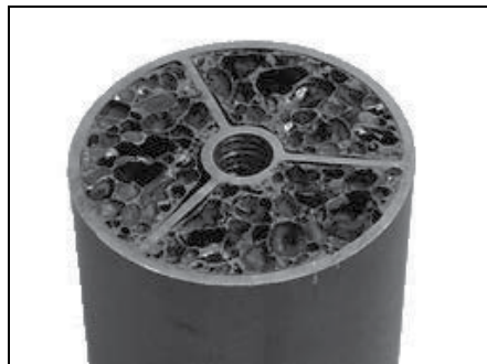
Fig. 3. Hollow tube filled with foam (courtesy of Valerio Mussi - MUSP)
