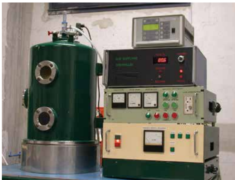
Fig. 1. The scheme of the system used for deposition of hard carbon coatings by PACVD method
