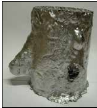
Fig. 10. MGI foam core insert with spacers
