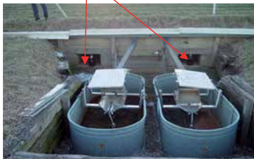
Figure 5. Pan lysimeters installed down the soil column (2 m deep) at the end of field plots for collection of infiltration water (Kentucky State University, Franklin County, KY).
