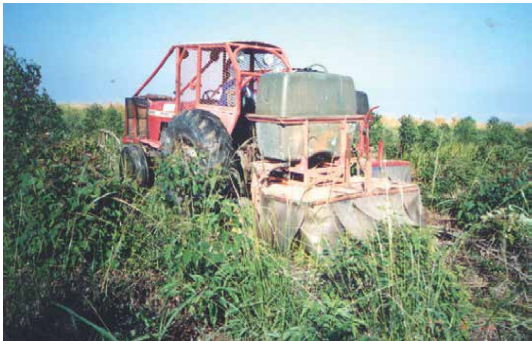
Figure 4. Sprayer bar protected with plastic blades attached to the bar used to apply nonselective herbicide between plant rows in eucalyptus plantation areas [24].
