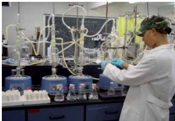
Figure 13. Use of soxhlet extraction units and liquid-liquid partition for extraction of dimethazone and trifluralin herbicides from soil.
