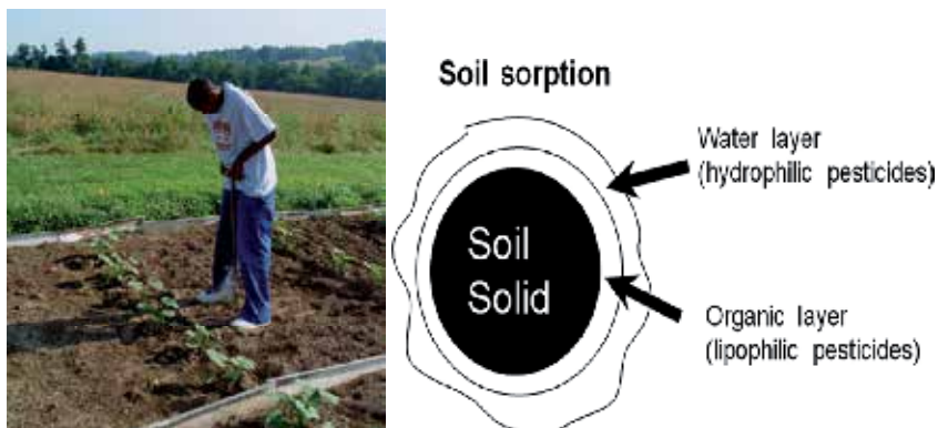
Figure 6. Collection of soil samples using a core sampler equipped with a plastic liner tube (left photo) and a schematic representation of sorption on soil particle (right sketch).
