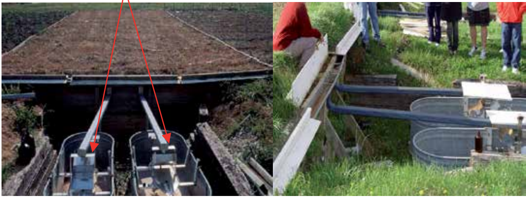
Figure 4. Surface runoff water collection using tipping buckets installed down the field slope. A gutter was installed across the lower end of each plot with 5% slope to direct runoff to the tipping buckets and collection bottles for runoff water measurement and sampling
