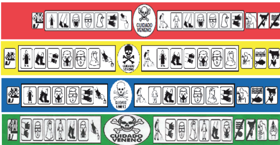
Figure 3. Warning band required at the bottom of the label, colored according to the toxicological class and pictograms about environmental and worker safety.
