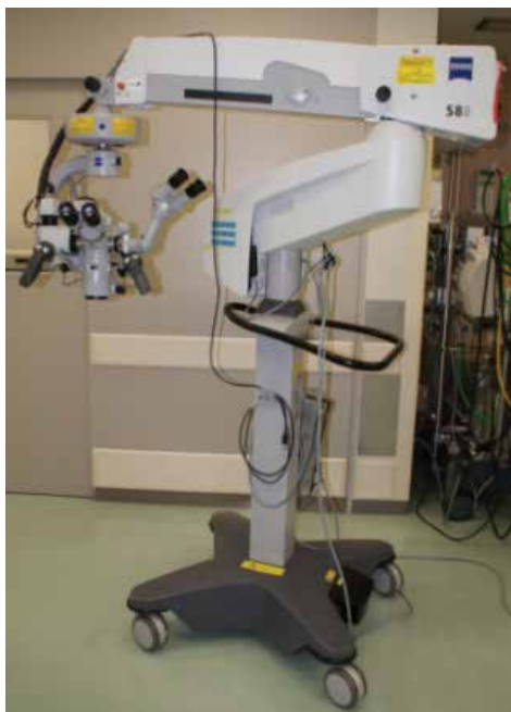
Fig. 4. The surgical microscope used for microvascular hepatic artery reconstruction (Carl Zeiss, OPMI VARIO S88). This microscope has a foot pedal. The surgeon can adjust the microscope using this foot pedal without interrupting the procedure
