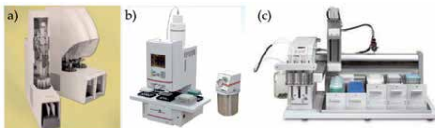
Figure 15. Most common robots for automated SPE (a) Zymark Rapid Trace System (b) Tomtec Quadra System (c) Gilson SPE 215 System.
