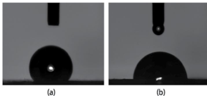
Figure 2. Water contact angle of (a) pure silk nanofibers; and (b) silk/TMOS nanofibers.
