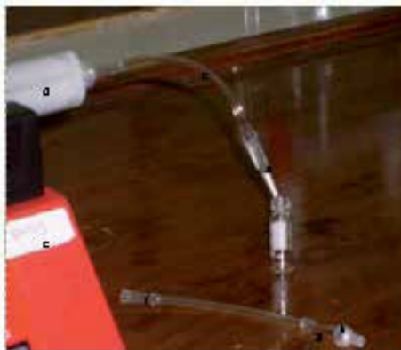
Figure 14. Syringe pump driven semi automated systems (a) micro column SPE device (b) modified disk (I) and disk (II) SPE device (s) (c) syringe pump (d) polypropylene syringe (e) PVC tubing (f) polypropylene adaptor (g) glass adaptor.
