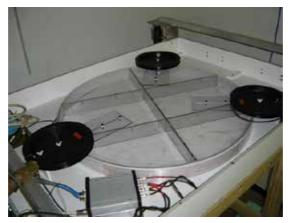
Fig. 14. The interior of the coil module showing the one-meter diameter transmit coil and the three separate receive coils.
