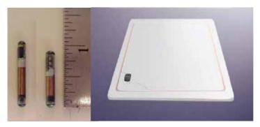
Fig. 2. Two examples of the low-frequency passive tags. The photo on the left shows the solenoid tag design; the coil wire is wrapped around a small permeable core. The photo on the right shows the "pancake" coil design used in non-contact facility access applications. The small black objects in the figures are the integrated circuits.
