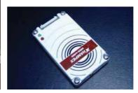
(c) The UHF RFID with casing (d) The portable UHF RFID readers tag(CONFIDEX STEELWAVE used in the experiment.
