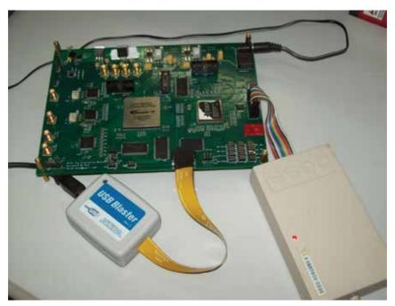
Fig. 11. Tag simulator main circuit board
