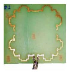
Fig. 27. The Fabricated Fractal Loop Antenna.
