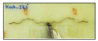
Fig. 9. Photograph of the fabricated K3-27.5° antenna.
