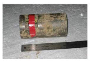
Fig. 15. Munition surrogate later buried at Aberdeen Test Center. The tag is evident below the red tape.
