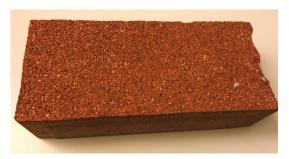
Figure 2. Photocatalytic concrete pavement block.
