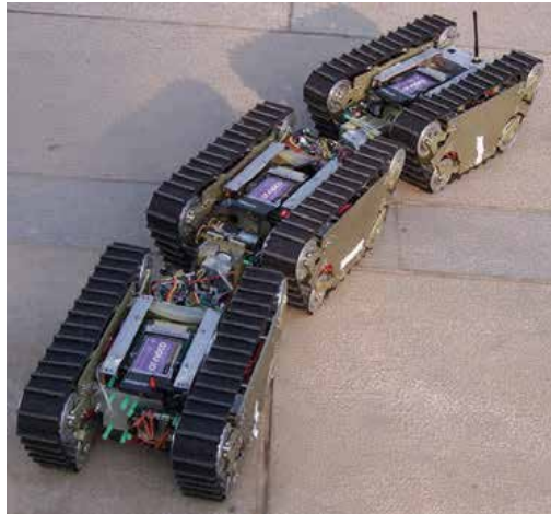
Fig. 12. Reconfigurable robot JL-I developed by Zhang et al. (2006)
