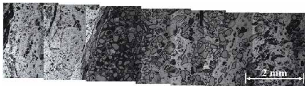
Fig. 5. Metallographic section of the Tantura F Anchor A corrosion layer (left) and the encrustation coating that includes sand particles (center and right) (Photos: D. Ashkenazi).
