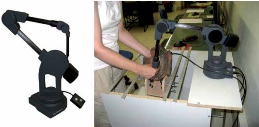
Fig. 9. Picture of a 3D Microscribe Digitizer (left) and view example of its employment (right).
