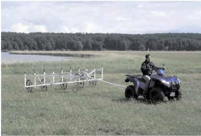
Fig. 12. A stack of magnetic gradiometers built by Eastern Atlas for large area surveys. Image courtesy of Cornelius Meyer.
