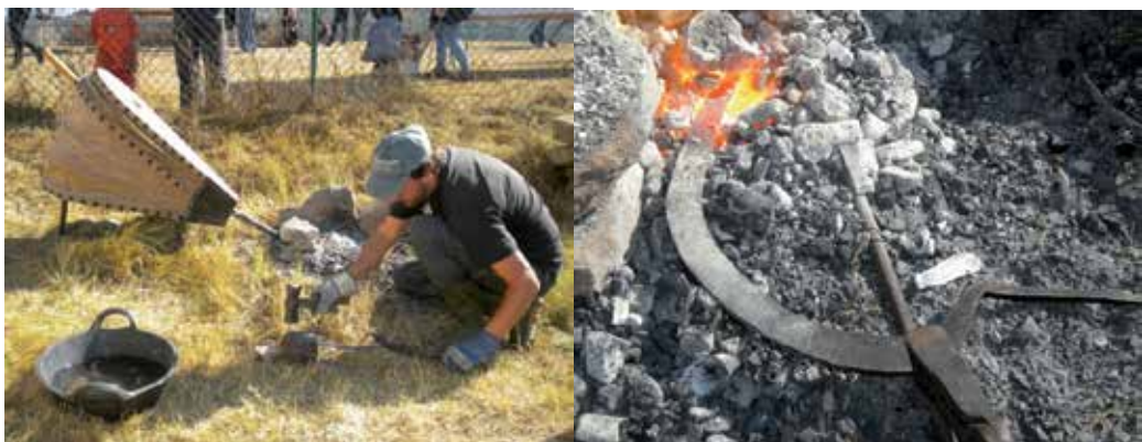
Fig. 16. Experimental process of an iron sickle forging and production
