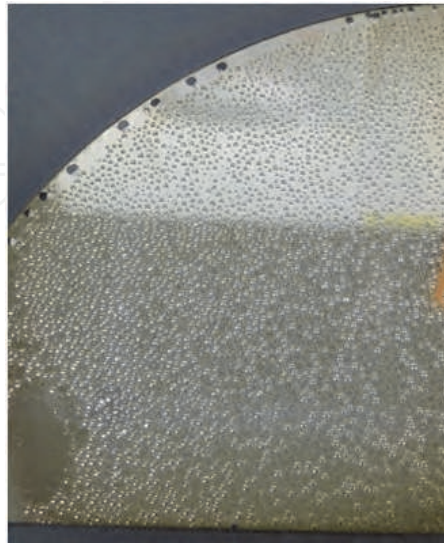
Fig. 16. Photo of the impact of pure argon etch on silver
