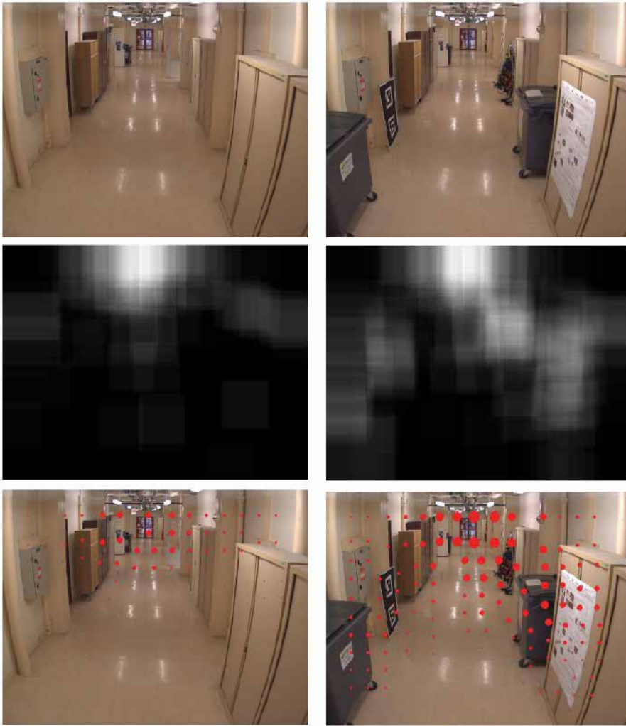
Fig. 16. Sampling grid in the case of calibration in a corridor. The first row shows the scene observed by the static camera. The second row represents the estimate of the probability density of SIFT points using Parzen windows. The last row shows the obtained sampling grid (the circles size is related to the probability density of the interest point).
