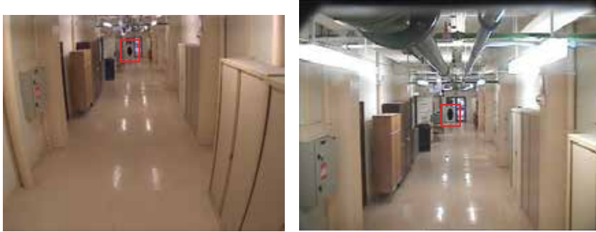
Fig. 11. Illustration of the elliptic calibration pattern (surrounded by red) used to evaluate the accuracy of the method of calibration. Left: in the static camera, right: in the dynamic camera.
