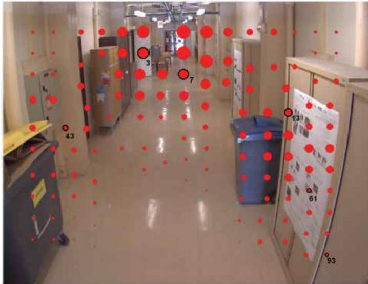
Fig. 12. Learning grid for calibration. The points surrounded by black are used in the discussion on the accuracy of the calibration. The size of the circles represents the probability density of detected SIFT points.
