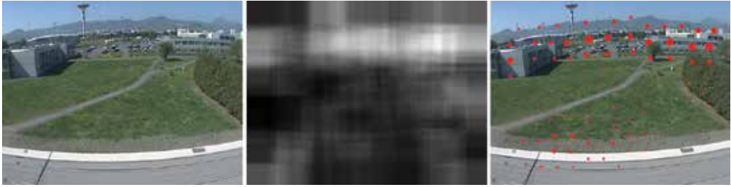
Fig. 10. Adaptive grid sampling of the 3-D scene. Left: the source image, middle: image representing the probability density of interest points using the Parzen windowing technique, right: the obtained sampling grid. The size of red circles represents the probability of the node.
