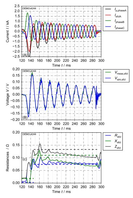
Figure 5.22: Results for fault current limitation of a 3-phase fault with ground connection for (a) currents, (b) voltages and (c) resistances ( $S_{\text{base}}$  = 180 kVA,  $R_{\text{fit}}$  = 40 m $\Omega$ ,  $p_{\text{f}}$  = 1.0)
