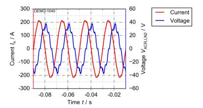
Figure 4.27: Measured current and voltage drop across the primary winding at 77 K during normal operation
