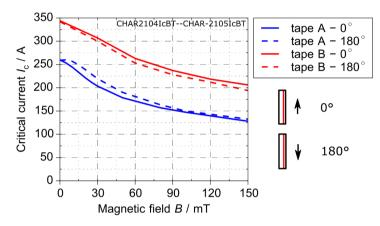
Figure 4.4: Measured critical current I<sub>c</sub> depending on magnetic field density for parallel field
