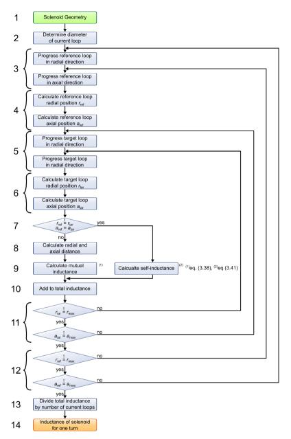
Figure B.1: Flow diagram of the function to calculate the inductance of a solenoid with arbitrary cross section
