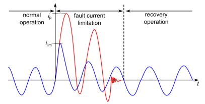
Figure 2.9: Operational modes of a superconducting fault current limiter. The red curve shows the unlimited fault current and the blue curve the limited fault current
