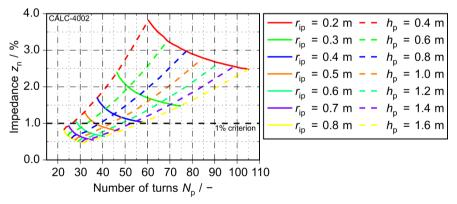
Figure 6.3: Calculated impedance during normal operation of 10 kV,1 kA, z = 6% AC-SFCLs for variation of the geometry of the primary winding
