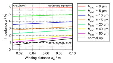
Figure 6.11: Dependency of the calculated impedance on winding distance and stabilization for the low impedance design (*I*<sub>max</sub> =300 A)
