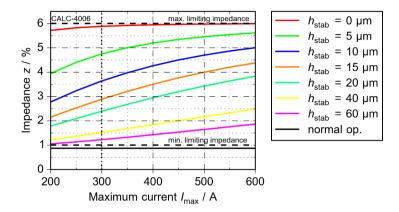
Figure 6.12: Dependency of the calculated impedance on critical current and stabilization for the low impedance design ( $d_w = 3 \text{ cm}$ )
