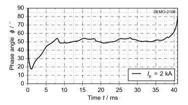
Figure 4.32: Calculated phase angle between current and voltage for the fault of four cycles shown in Figure 4.29
