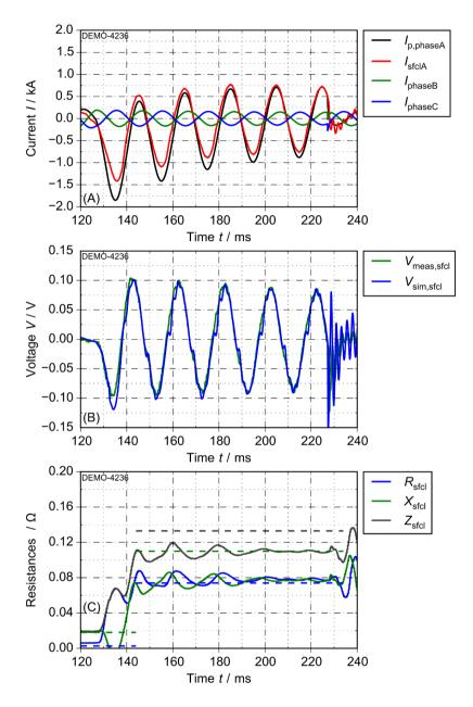
Figure 5.16: Results for fault current limitation of a 1-phase fault for (A) currents, (B) voltages and (C) resistances ( $S_{\text{base}}$  = 120 kVA,  $R_{\text{fit}}$  = 40 m $\Omega$ ,  $p_{\text{f}}$  = 1.0)
