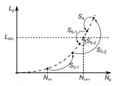
Figure 3.10: Iterative approach to calculate the inductance  $L_p$  of the primary winding The number of turns is varied in discrete steps until the calculated impedance  $L_p$  matches the impedance necessary for fault current limitation
