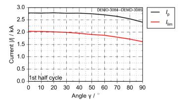
Figure 4.36: Measured fault limitation capability for a fault angles between 0° and 90° in the first half cycle
