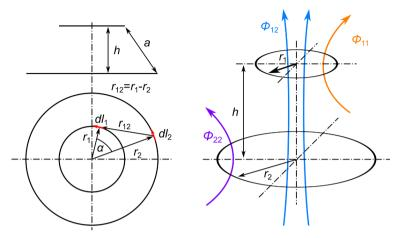
Figure 3.5: Two coaxial current loops with radii r<sub>1</sub> and r<sub>2</sub> and distance h
