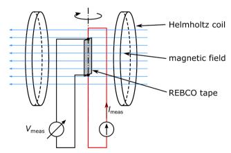
Figure 4.3: Schematic of the setup for measuring the critical current *l<sub>c</sub>*(*B*,*T*). A homogeneous magnetic field is generated using two Helmholtz coils. he *RE*BCO tape is rotated within the magnetic field.
