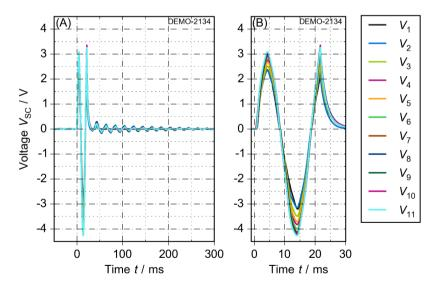
Figure 4.39: Voltage signals at the *RE*BCO tapes during fault current limitation for a fault of two half cycles (A) including the load cycle and (B) magnified on the fault.
