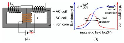
Figure 2.11: (A) Schematic of the saturated iron core SFCL for single phase and (B) qualitative magnetization curve with regions of operation according to [MD09]
