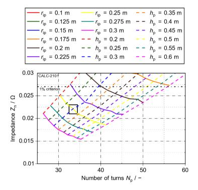
Figure 4.18: Results for impedance during normal operation of the demonstrator in the first design step magnified on geometries fulfill the  $z \le 1\%$  criterion (fill-factor  $f_{\rm fp}$  = 0.85). The rectangle indicates the chosen geometry
