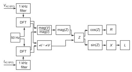
Figure 5.9: Approach to calculate instantaneous values of resistance and inductance from measured voltage and current
