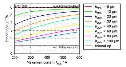
Figure 6.2: Calculated impedance of the retrofit for normal operation and fault condition for constant winding distance  $d_w = 2 \text{ cm}$
