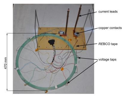
Figure 4.8: Mechanical setup for measuring the critical current at self-field and 77 K. The *RE*BCO tape is bend with the same diameter as in the AC-SFCL.
