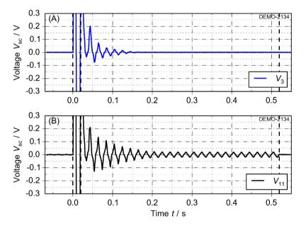
Figure 4.41: Voltages of two *REBCO* tapes during fault and following load cycle. (A) shows the recovery of tape 3, which recovers 124 ms after the fault is switched of, while in case (B) the tape is not recovering
