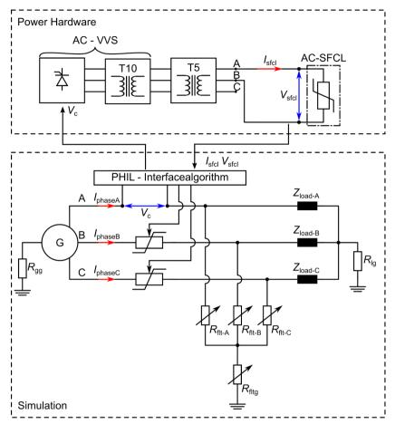
Figure 5.15: Three phase PHIL test setup. The Hardware part remained the same as in the preliminary tests shown in Figure 5.4
