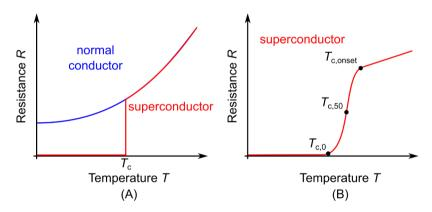
Figure 2.1: (A) Resistance depending on temperature for superconductors and normal conductors and (B) magnification around the transition and different definitions of the critical temperature [Cav98]
