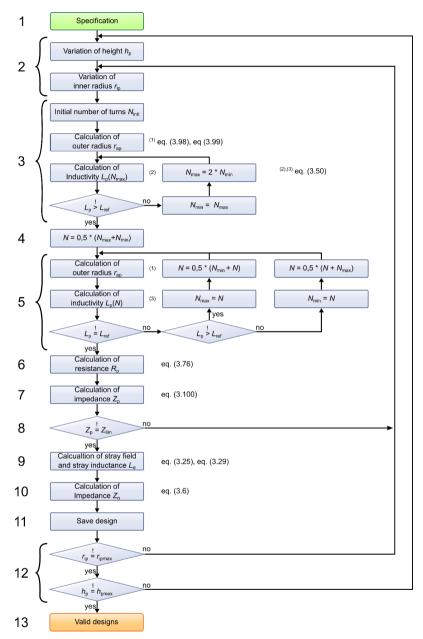
Figure 3.11: Flow diagram for optimized design. With a set of geometrical parameters the number of turns *N* are calculated to match the reference impedance *L*<sub>ref</sub> and the impedance *Z*<sub>lim</sub> assuming constant parameters for secondary winding.
