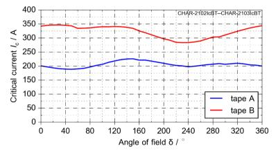
Figure 4.6: Measured critical current  $l_c$  depending on the angle of the magnetic field for tape A and tape B for a magnetic field density of B = 30 mT
