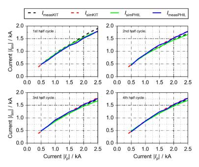
Figure 5.7: Comparison of PHIL results with KIT results for fault current limitation during four half cycles for increasing prospective currents. The example shown in Figure 5.5 is indicated.
