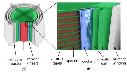
Figure 2.14: Schematic of the AC-SFCL: (A) Air core reactor with insert and (B) magnification of the insert showing the insulation and the winding
