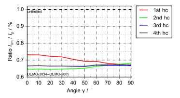
Figure 4.37: Measured fault current limitation for a fault angles y between 0° and 90° for all four half cycles
