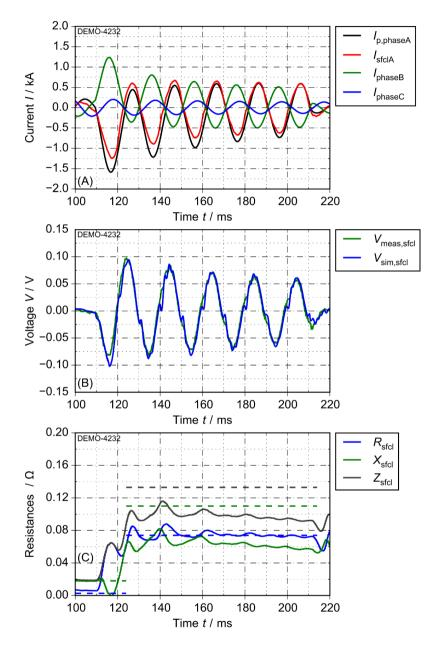
Figure 5.19: Results for fault current limitation of a 2-phase fault without ground connection for (A) currents, (B) voltages and (C) resistances (S<sub>base</sub> = 120 kVA, R<sub>fit</sub> = 40 mΩ, p<sub>f</sub> = 1.0)
