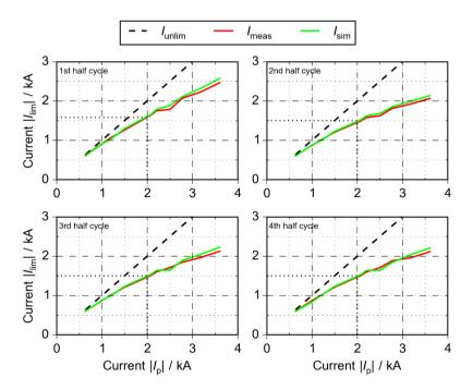
Figure 5.3: Comparison of the simulated model and measured results at KIT for fault current limitation for a fault currents with increasing prospective current (the example in Figure 5.2 is indicated)
