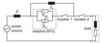
Figure 2.10: Circuit diagram of a resistive type SFCL with parallel impedance Z<sub>s</sub> and circuit breakers
