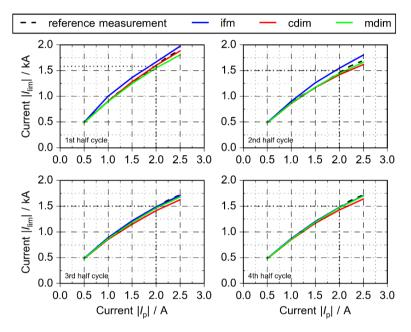
Figure 5.13: Comparison of current limitation of the three interface algorithms - simulation
