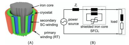
Figure 2.12: (A) Schematic of the shielded iron core SFCL and (B) equivalent circuit diagram
