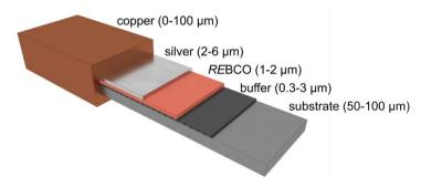
Figure 2.5: Typical layered structure of a *RE*BCO conductor. Thickness and width of the layers are not to scale
