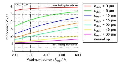
Figure 6.18: Dependency of the calculated impedance on critical current and stabilization for the low impedance design ( $d_w = 10$  cm)
