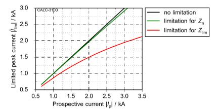
Figure 4.24: Simulation of expected progression of peak limited short-circuit current  $|\hat{l}_{lim}|$  with peak prospective current  $|l_{p.}|$ . The example in Figure 4.23 is indicated.
