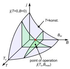
Figure 2.4: Combination of all three critical values to determine the point of operation with safety margins according to [Kom95]
