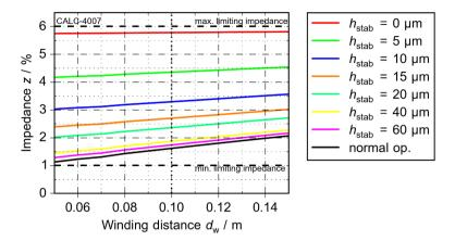
Figure 6.14: Calculated impedance of the retrofit for normal operation and fault condition for constant current *I*<sub>max</sub> = 300 A
