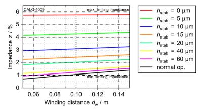
Figure 6.17: Dependency of the calculated impedance on winding distance and stabilization for the low impedance design (*I*<sub>max</sub> = 300 A)
