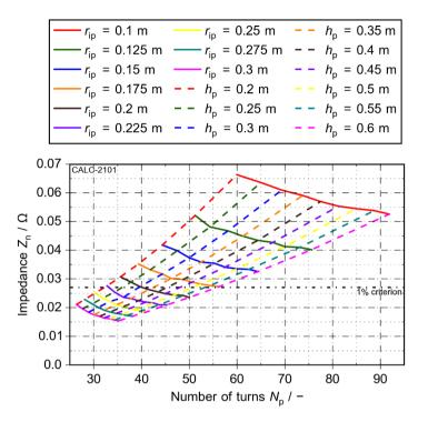
Figure 4.17: Results for impedance during normal operation of the demonstrator in the first design step (fill-factor  $f_{fp}$  = 0.85)
