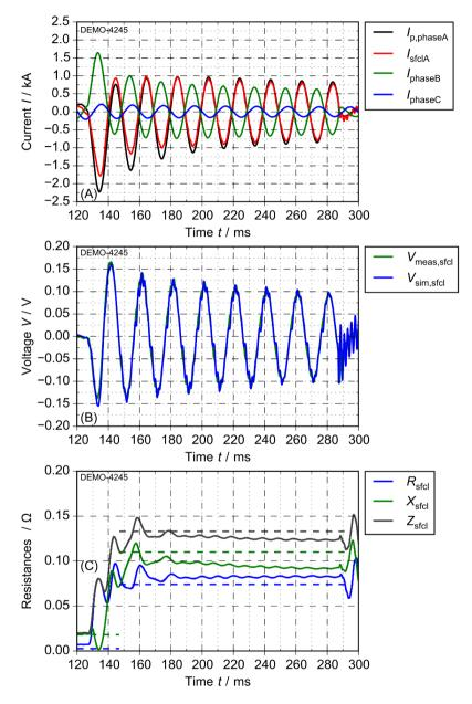
Figure 5.21: Results for fault current limitation of a 2-phase fault with ground connection for (a) currents, (b) voltages and (c) resistances ( $S_{\text{base}}$  = 180 kVA,  $R_{\text{fit}}$  = 40 m $\Omega$ ,  $p_{\text{f}}$  = 1.0)
