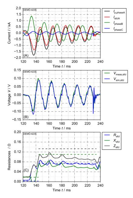
Figure 5.17: Results for fault current limitation of a 2-phase fault with ground connection for (A) currents, (B) voltages and (C) resistances ( $S_{\text{base}} = 120 \text{ kVA}$ ,  $R_{\text{flt}} = 40 \text{ m}\Omega$ ,  $p_{\text{f}} = 1.0$ )
