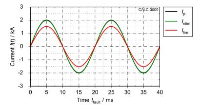
Figure 4.23: Simulation of an expected fault current limitation of the AC-SFCL demonstrator. A prospective short-circuit current of  $I_p$  = 2 kA is limited to  $I_{lim}$  = 1.5 kA
