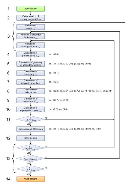
Figure 3.9: Flow diagram for calculation of the retrofit. Assuming constant parameters for the primary winding a secondary winding is calculated. If the impedance of the design during normal operation the AC-losses of the AC-SFCL design are calculated and the design is stored.
