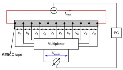
Figure 4.7: Setup to measure critical current distribution of each *RE*BCO tape intended for the use in the AC-SFCL demonstrator. The current is increased in discrete steps and the voltage drop of each section is measured after each current increase.
