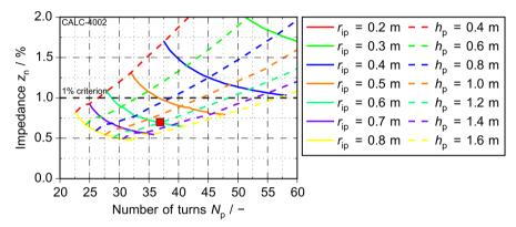
Figure 6.4: Magnified view of Figure 6.3. The red square indicates the chosen low impedance design
