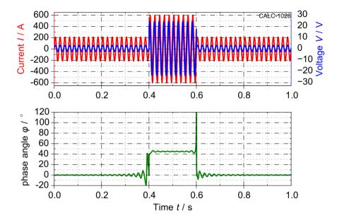
Figure C.4: Load-fault-load cycles. The phase angle between voltage and current is  $\varphi = 0^{\circ}$  during load and  $\varphi = 45^{\circ}$  during fault
