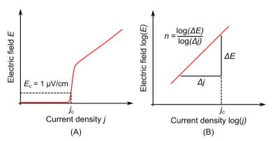
Figure 2.2: (A) Definition of the critical current density  $j_c$  and (B) definition of the n-value
