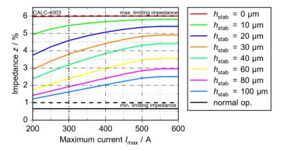
Figure 6.6: Dependency of impedance on critical current and stabilization for the low impedance design ( $d_w = 2 \text{ cm}$ )
