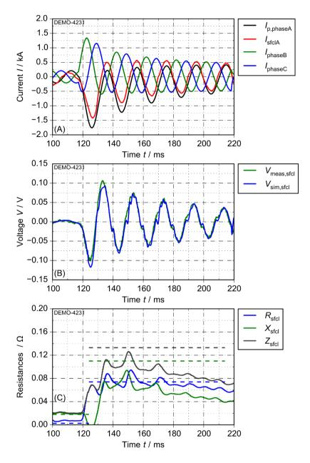
Figure 5.20: Results for fault current limitation of a 3-phase fault without ground connection for (A) currents, (B) voltages and (C) resistances (S<sub>base</sub> = 120 kVA, R<sub>fit</sub> = 40 mΩ, p<sub>f</sub> = 1.0)
