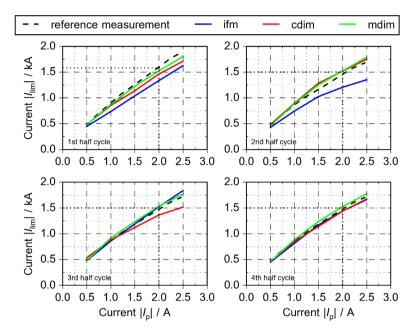
Figure 5.14: Comparison of current limitation of the three interface algorithms - measurement
