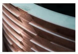
Figure 4.21: Close-up of the secondary winding. The *RE*BCO tapes can be identified by their brushed copper surface. Spacers between the *RE*BCO tapes keep the tapes separated and at position, while the cuttings in the spacers allow the flow of liquid nitrogen.
