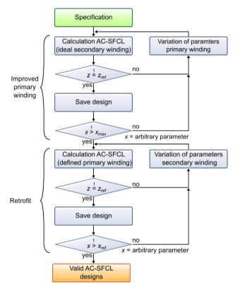
Figure 3.8: General approach of the proposed design method. The design process is separated into two major parts, the calculation of a design with an improved primary winding and the insert. This allows independent the calculation of the retrofit of an air core reactor and the design of an AC-SFCL with improved primary winding.
