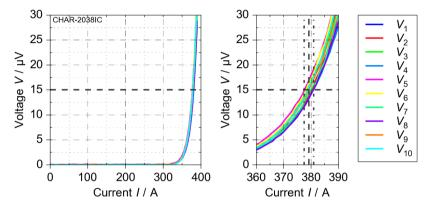
Figure 4.10: Measurement of critical current *I*<sub>c</sub> for a sample of tape B at self-field
