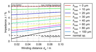
Figure 6.5: Dependency of impedance on winding distance and stabilization for the low impedance design (*I*<sub>max</sub> = 300 A)
