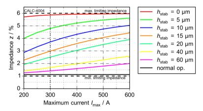
Figure 6.9: Calculated impedance of the retrofit for normal operation and fault condition for constant winding distance  $d_w = 3$  cm
