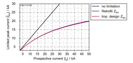
Figure 6.13: Expected fault current limitation of the retrofit and the low impedance design for 110 kV, 1 kA, z = 6%
