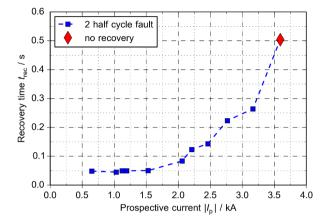
Figure 4.42: Summarized results of recovery under load. At  $|I_p| = 3.6$  kA the tape shown in Figure 4.41 is not recovering
