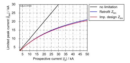
Figure 6.19: Expected fault current limitation of the retrofit and the low impedance design for 380 kV, 1 kA, z = 6%
