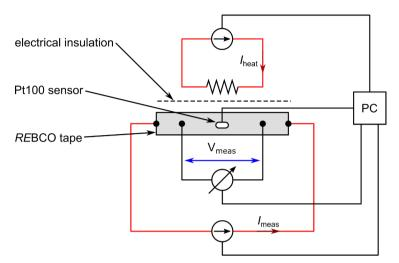
Figure 4.1: Diagram of the setup to measure the resistance depending on temperature R(T). The *REBCO* tape is cooled down to 77 K and the slowly heated up. During the heating process a small current  $I_{meas}$  and the voltage drop across the tape  $V_{meas}$  are used to calculate the resistance R(T).
