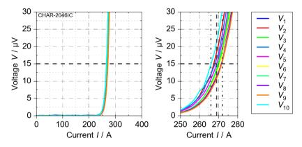
Figure 4.9: Measurement of critical current *I*c for a sample of tape A at self-field
