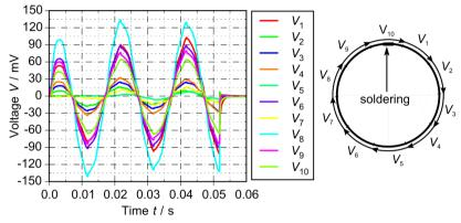
Figure 4.16: Quench results of a single short-circuited *RE*BCO ring (tape B) with ten voltage taps (order is shown on the right)
