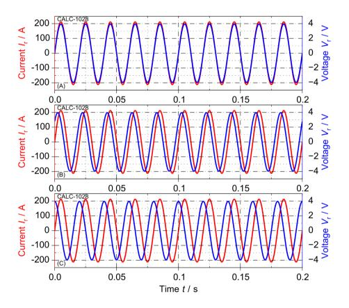
Figure C.1: Generated sine signals for voltage and current with phase angles of (A) 0°, (B) 45° and (C) 90°
