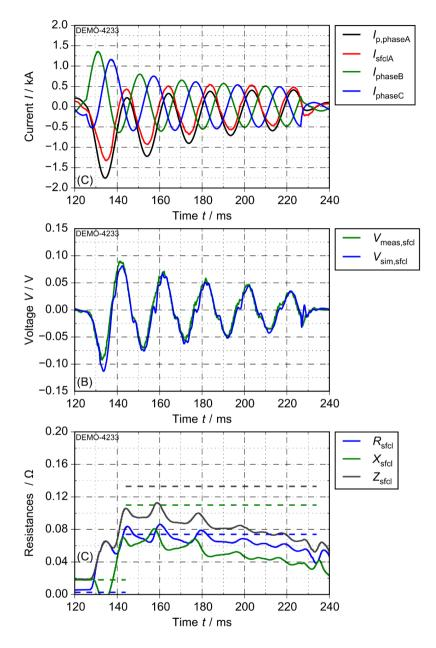
Figure 5.18: Results for fault current limitation of a 3-phase fault with ground connection for (A) currents, (B) voltages and (C) resistances ( $S_{\text{base}}$  = 120 kVA,  $R_{\text{ft}}$  = 40 m $\Omega$ ,  $p_{\text{f}}$  = 1.0)
