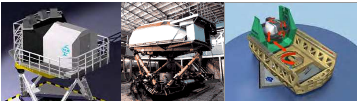
Fig. 16. SUPRA simulation facilities for conducting advanced upset recovery simulation research to improve pilot training in upset recovery and reduce LOC-I accident rates. Left: NLR Generic Research Aircraft Cockpit Environment (GRACE). Mid: TsAGI PSPK-102. Right: TNO/AMST Desdemona
