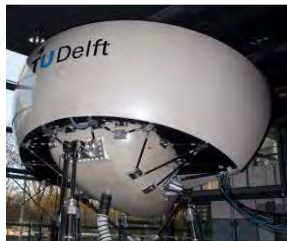
Fig. 12. Evaluation of GARTEUR FM-AG(16) FTFC techniques in the Delft University SIMONA Research Simulator based on reconstructed accident scenarios (Left: Boeing 747 cockpit configuration. Right: visual system dome)
