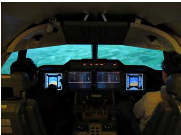
Fig. 12. Evaluation of GARTEUR FM-AG(16) FTFC techniques in the Delft University SIMONA Research Simulator based on reconstructed accident scenarios (Left: Boeing 747 cockpit configuration. Right: visual system dome)
