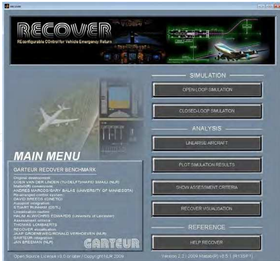
Fig. 9. GARTEUR RECOVER Benchmark graphical user interface for the selection of simulation and analysis tools
