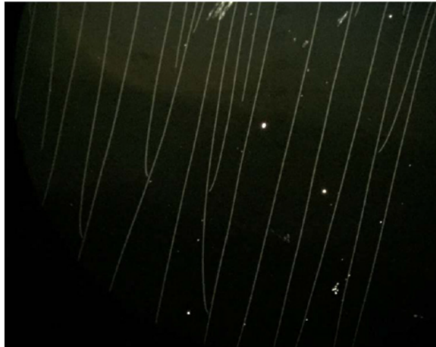
Figure 21. Cracks observed on an IBS \text{Ta}_2\text{O}_5\text{-ZrO}_2 thin film (LMA) after annealing at T_a = 700^\circ\text{C} .
