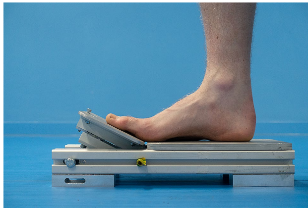
Figure 2. Image showing foot position on the dynamometer.
