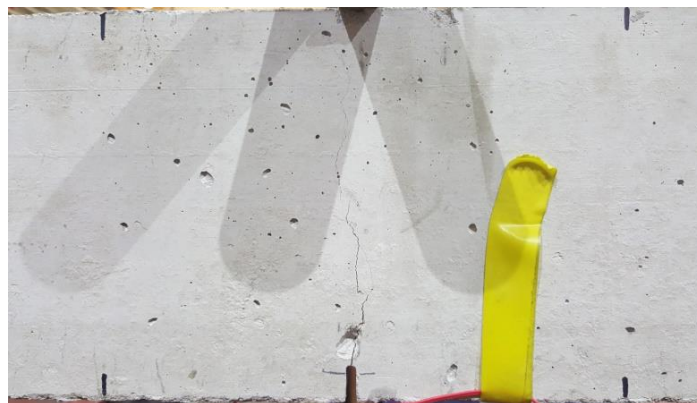
Figure 3-8. Final failure mode of the specimen in bending test
