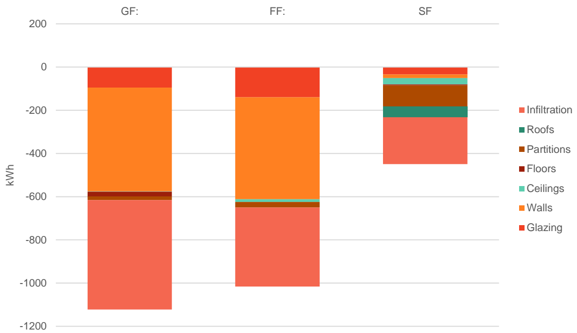
Elemental fabric heat losses by floor for pre-retrofit model of Test House B
