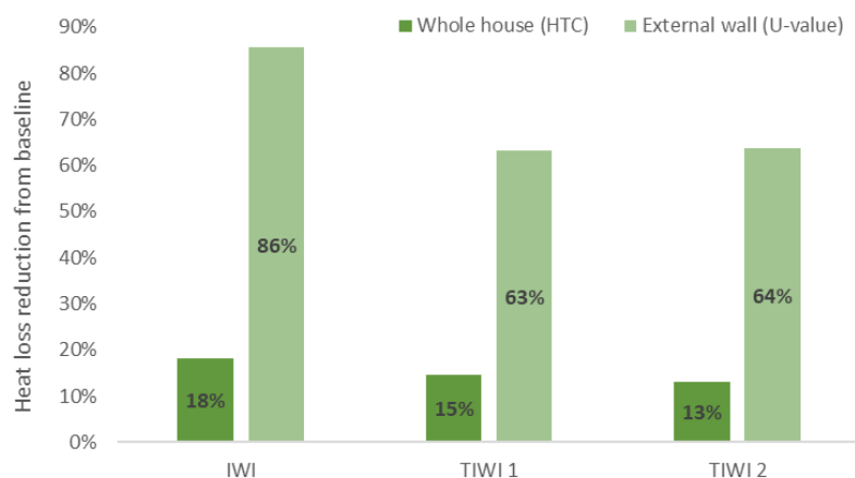
Figure 4-2 House A: Percentage reduction in HTC and external wall U-value resulting from each external wall retrofit measure
