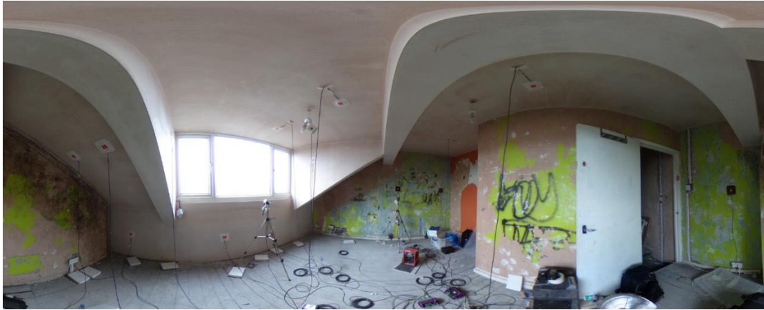
Figure 7-13 Experimental set-up in the TIWI over-boarded RiR (red disks are the HFPs)
