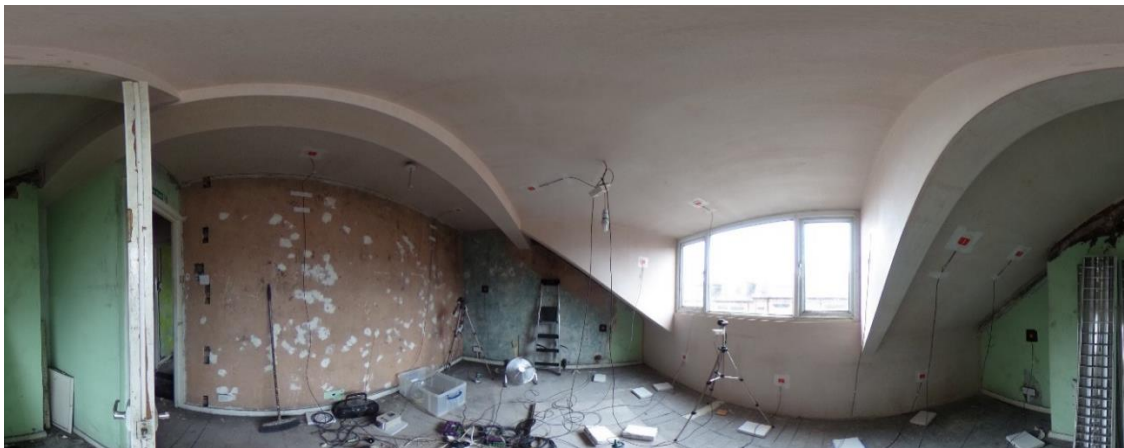
Figure 7-14 Experimental set-up in the conventionally retrofitted RiR (red disks are the HFPs)
