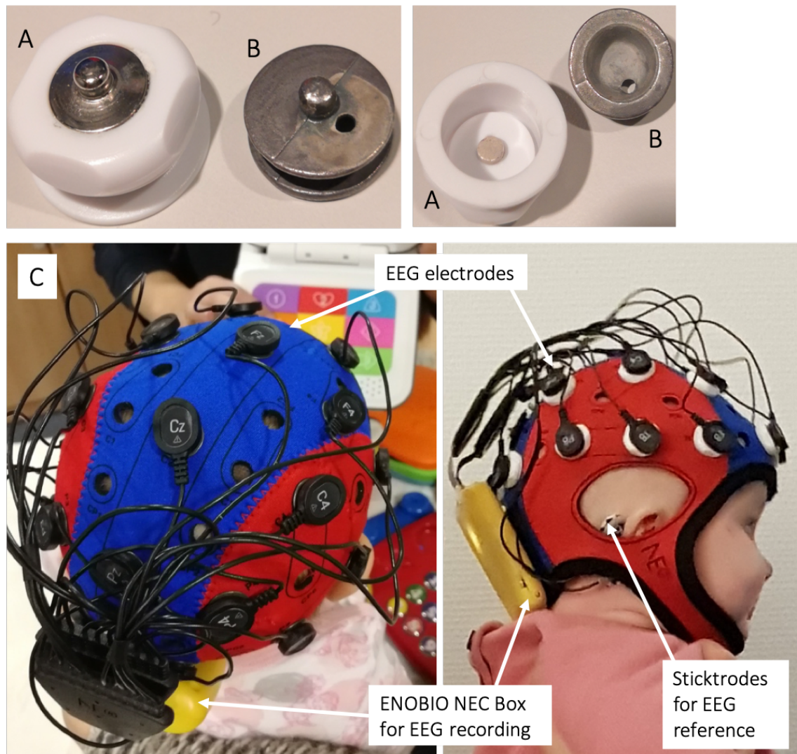
Figure 2.9. Illustration of the EEG electrodes used in Study 1 (electrode A) and Study 2 (electrode B). And an illustration of the wireless EEG system used in Study 1, that was later adapted for Study 2 and integrated with NIRS optodes (C).
