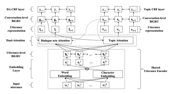
**Figure 3.1:** Overview of the dual-attention hierarchical recurrent neural network with a CRF.
