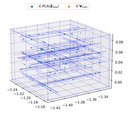
**Figure 5.1:** A cubic fence C in the latent space of Vanilla-VAE trained on the Wiki dataset, with  $d_r$  set at 3 to facilitate visualisation (cf. § 5.4). C, whose 12 edges are illustrated by dashed lines, surrounds the dimensionally reduced expectation of three encoded training samples. Traversed paths are illustrated by the solid lines within the cube.
