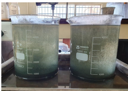
Figure 11—Settling of precipitants formed during the lime and soda ash treatment. The sample on the left was treated with unslaked lime, and that on the right was treated with a combination of unslaked lime and soda ash
