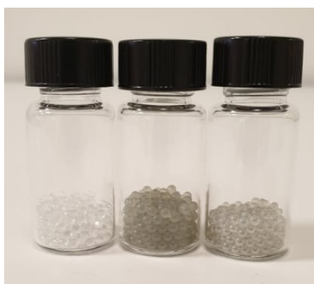
Figure 25 – Image of uncoated glass particulates (left,) as-deposited TiO 2 coated glass particulates (middle) and TiO 2 coated glass particulates annealed at 500°C (right).
