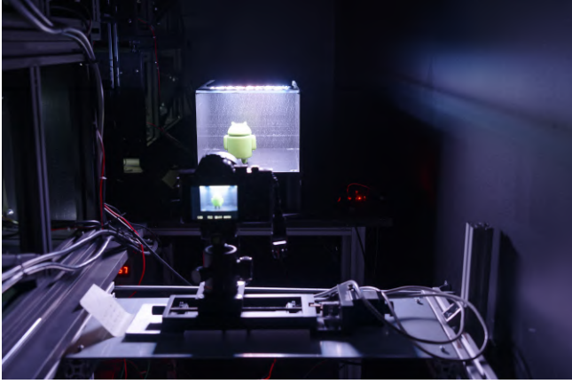
Fig. 8. The data camera and motorized slider for light field capture.
