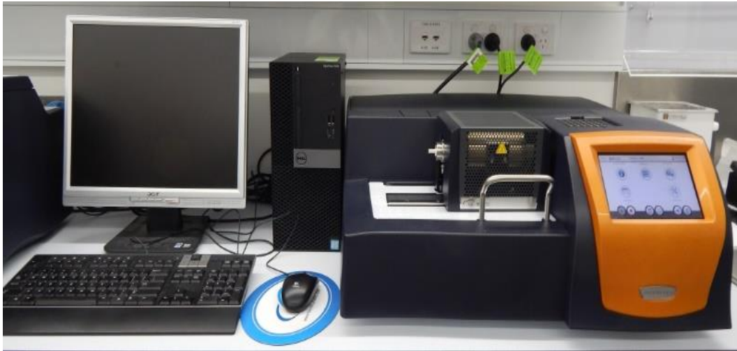
Fig. 6.8 TA SDT 650 (Discovery) model set up for TGA
