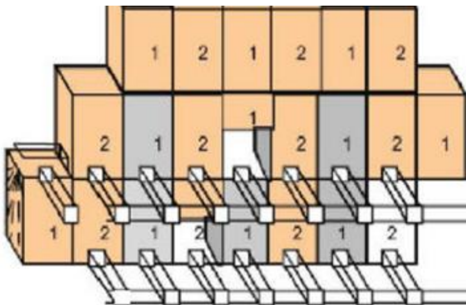
Fig. 2.4 Primary-secondary transverse in bulk hard rock (source: sec.gov)
