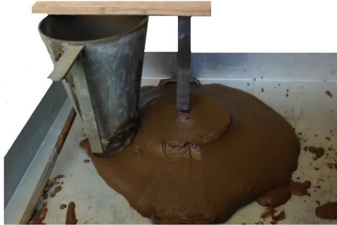
Fig. 7.7 Slump test of cemented paste fill
