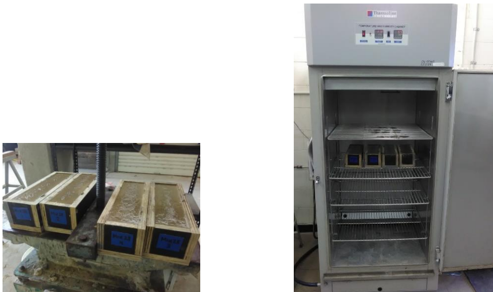
Fig. 5.19 Casting and storing 3-point samples
