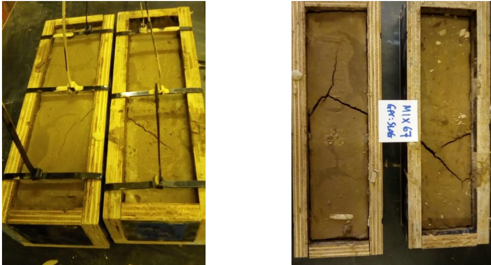
Fig. 5.22 Samples cracking with and without cable fasteners
