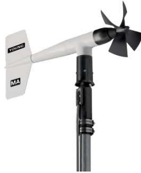
Figure 3.8. R.M Young Propeller Anemometer (Model 05106)
