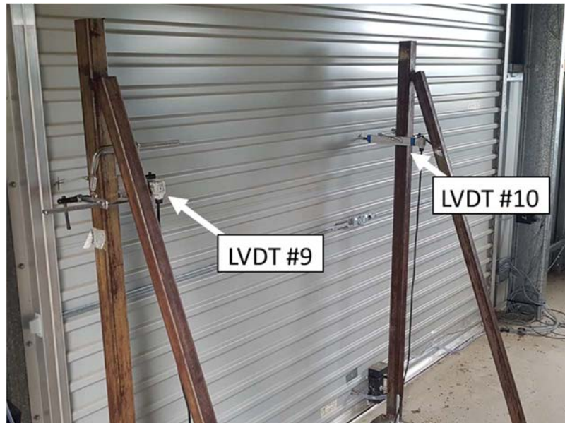
Figure 4.18. LVDT #9 and #10 mounted at edge and centre of the Western roller-door
