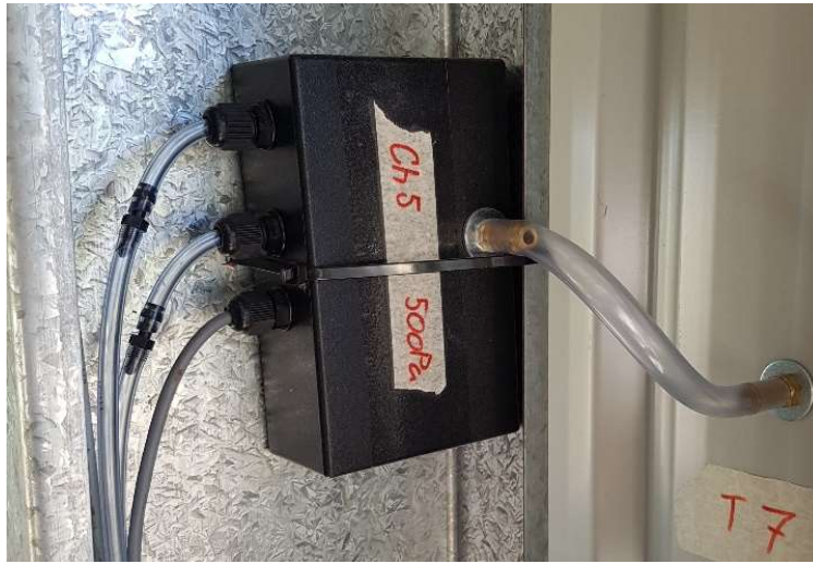
Figure B.5. Pressure transducer in situ connected tap T7 on the JCU-ASIS
