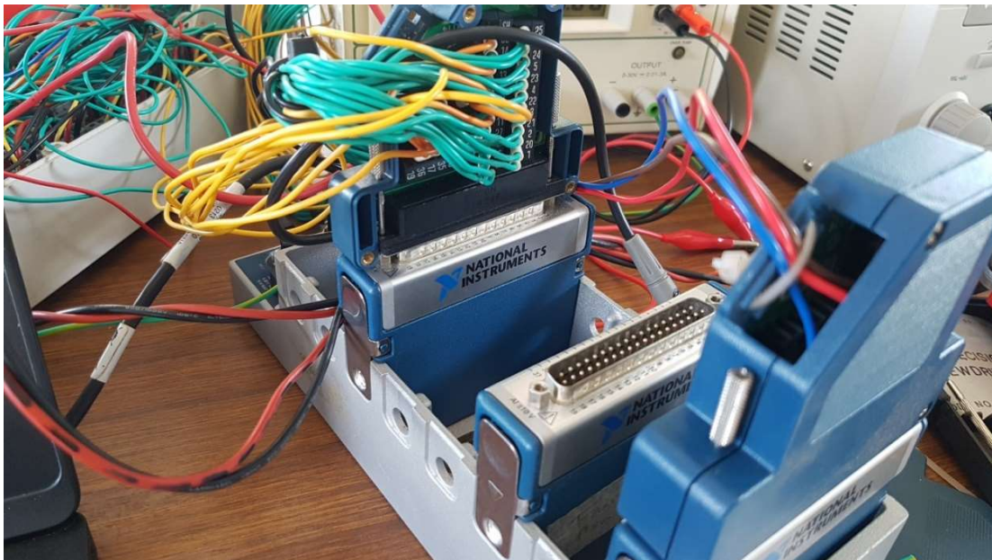
Figure B.1. Data acquisition system NI-cDAQ 9178 and input/output modules
