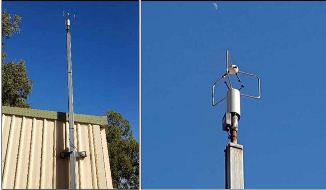
Figure 4.8. R.M. Young Ultrasonic anemometer on 5 m tall mast
