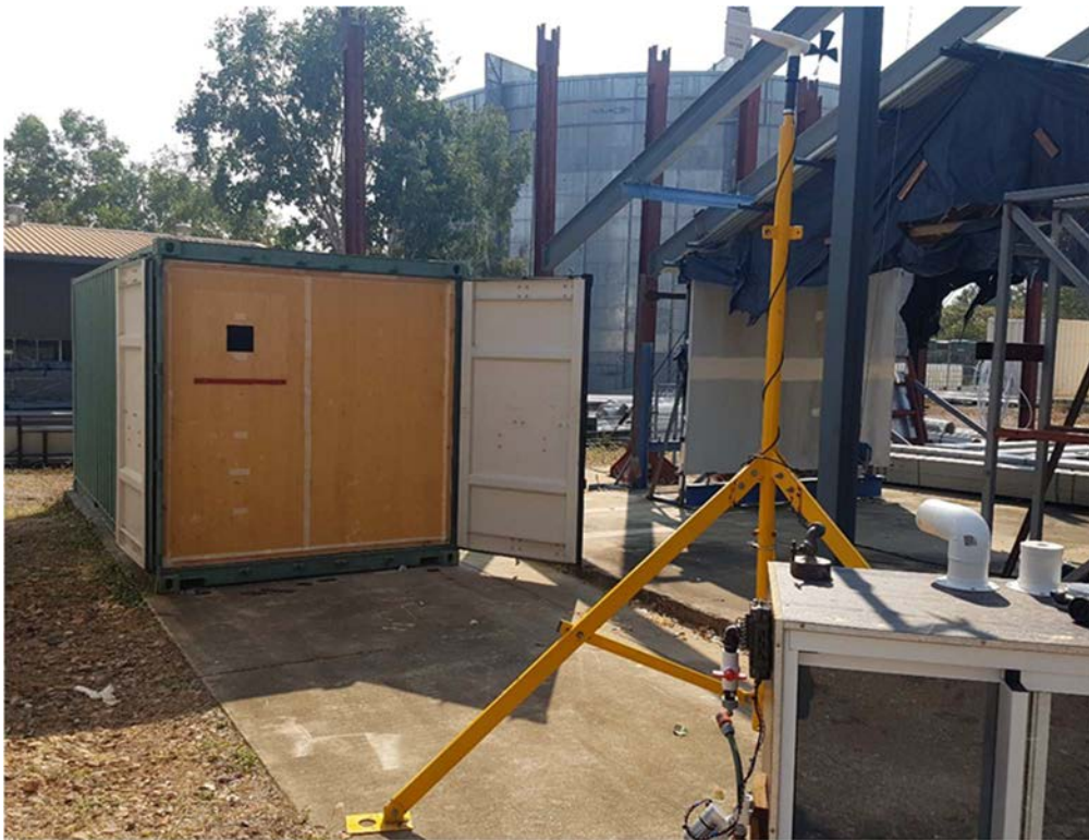
Figure B.8. FSTE during setup, (foreground) R.M. Young Anemometer 5 m from the FSTE, (background) Timber wall installed in FSTE.
