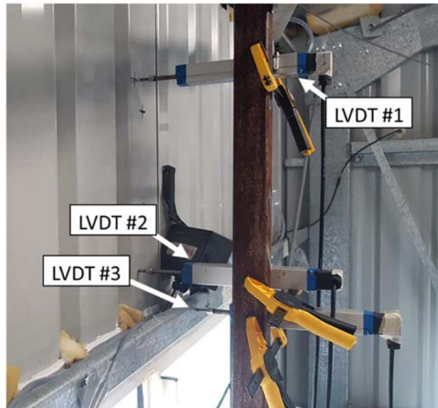
Figure 4.20. LVDT #1, #2, and #3, mounted on the Northern wall cladding and wall girt between Eastern and middle portal frames
