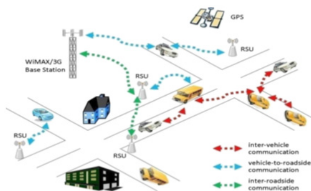
Fig1. Architecture of Vehicular Network.
