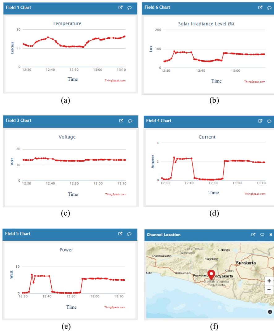
Figure 5. Captured visual data from ThingSpeak platform; (a) ambient temperature; (b) PV voltage out; (c) PV current out; (d) PV power out; (e) solar irradiance level; (f) channel location
