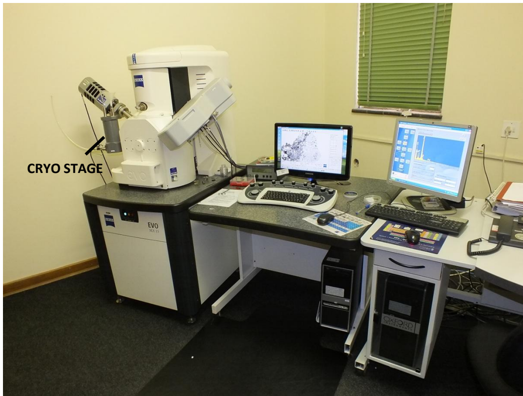
Figure 1.3 – Zeiss EVO@MA15 SEM with the cryostage coupled and the computers for the software for analyses. The samples were coated with carbon and loaded in the SEM with mineral standards for quantification. Backscatter images were also taking during analyses.
