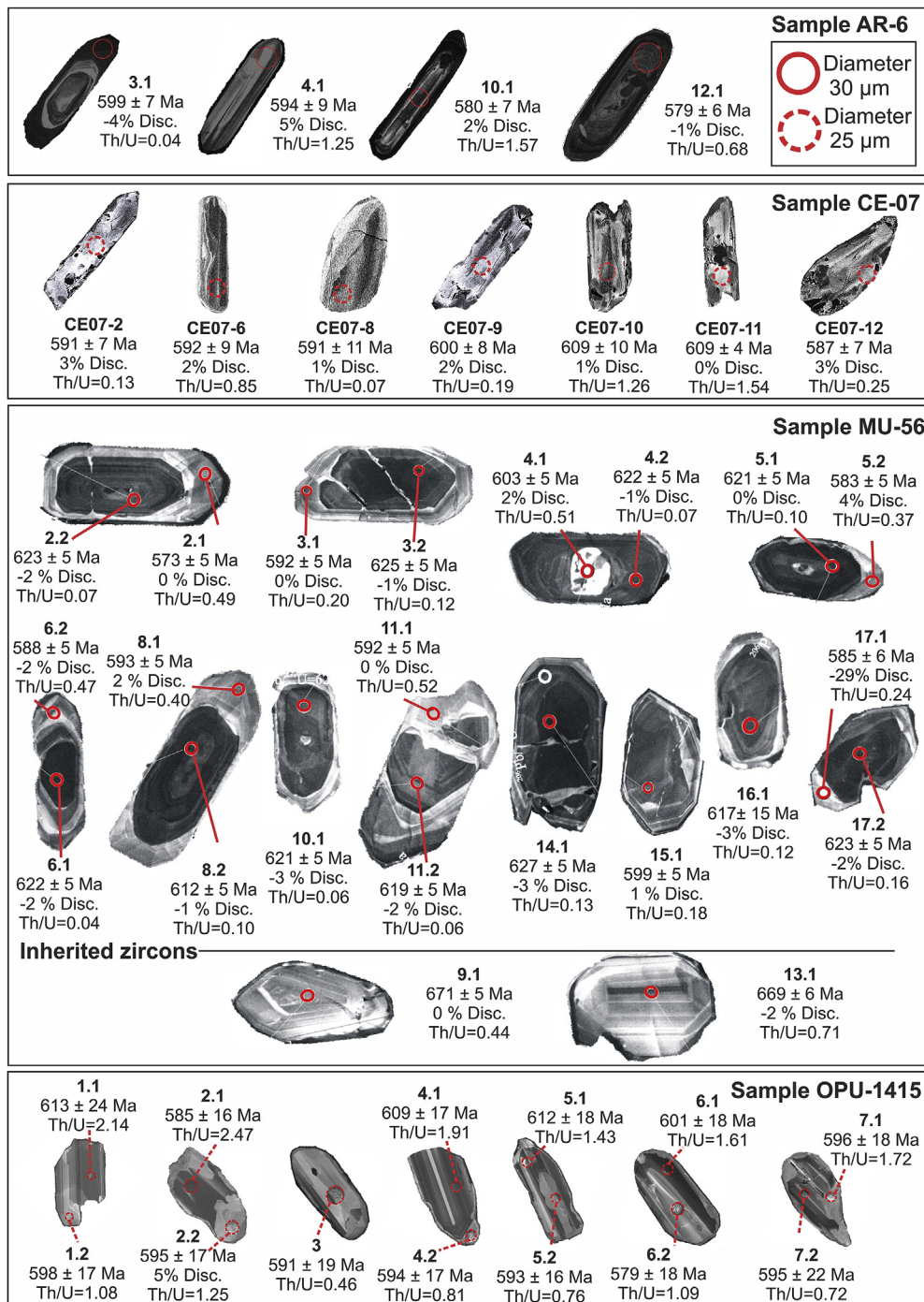
Fig. 10. Cathodoluminescence (CL) images of zircon grains from the Conceição da Boa Vista tonalitic orthogneiss (sample AR-6), migmatitic hornblende orthogneiss from the Muriaé batholith (sample MU-56), and metagabbro of the Serra do Valentim pluton (sample OPU-1415). Backscattered electron (BSE) images from zircon grains of the foliated granite from the Muriaé batholith (sample CE-07).
