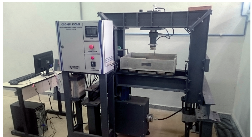
Figure 3 Large direct shear test equipment - UFOP Geotechnical Laboratory.
