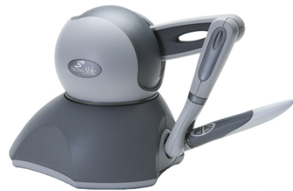
(b) The haptic device Phantom Omni (aka Geomagic Touch). Source: (THE. . . , 2017)
