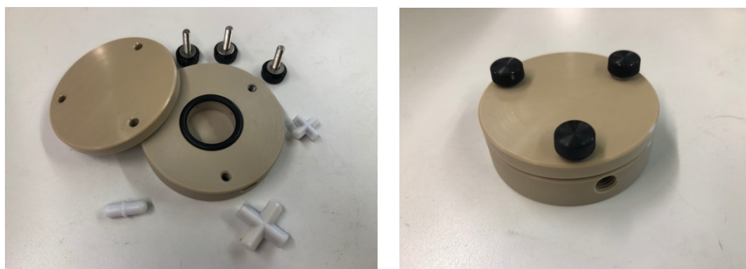
Figure 5.15. Self-made active mixing unit in open and closed form
