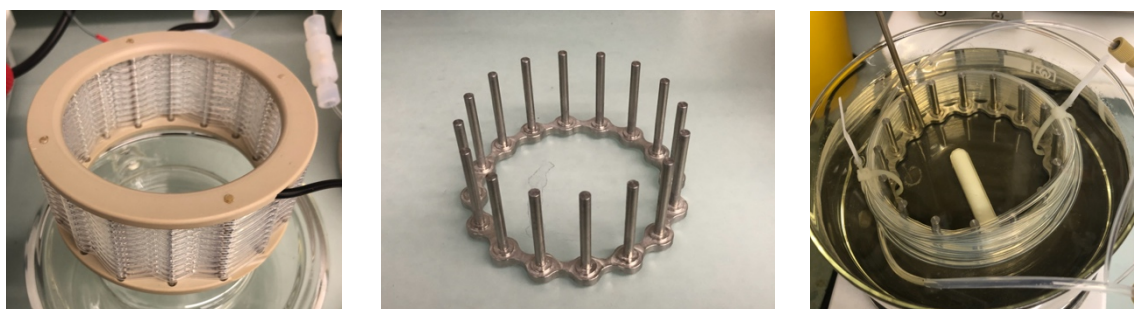
Figure 5.12. Left: commercial 10 mL reactor; middle: self-made stainless-steel holder; right: self-made 20 mL reactor immersed in oil bath
