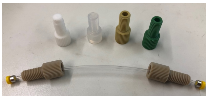
Figure 5.3. Back: Teflon® stopper (white), PCTFE (transparent) and PEEK (brown, green) fittings; front: assembly of FEP tubing with flangeless ETFE nuts (yellow) and PEEK fitting (beige)
