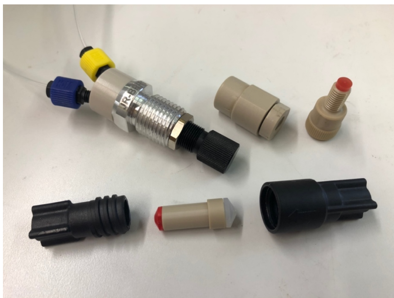
Figure 5.7. Top: adjustable back pressure regulator (left) and in-line check valves; Bottom: BPR assembly with preset back pressure cartridge
