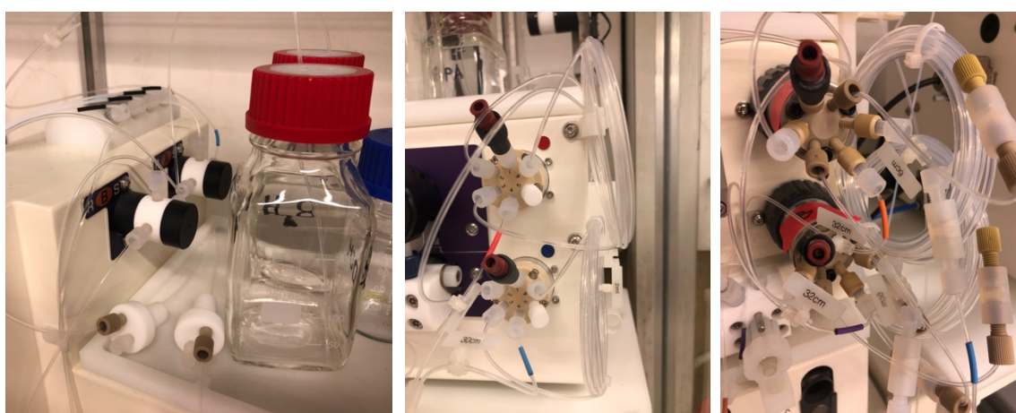
Figure 5.4. Left: bottled reagent and solvent connected to a T-shaped manifold; middle: 6-port manifold with 2 mL feeding loop; right: 6-port manifold with adjustable 10 mL feeding loop
