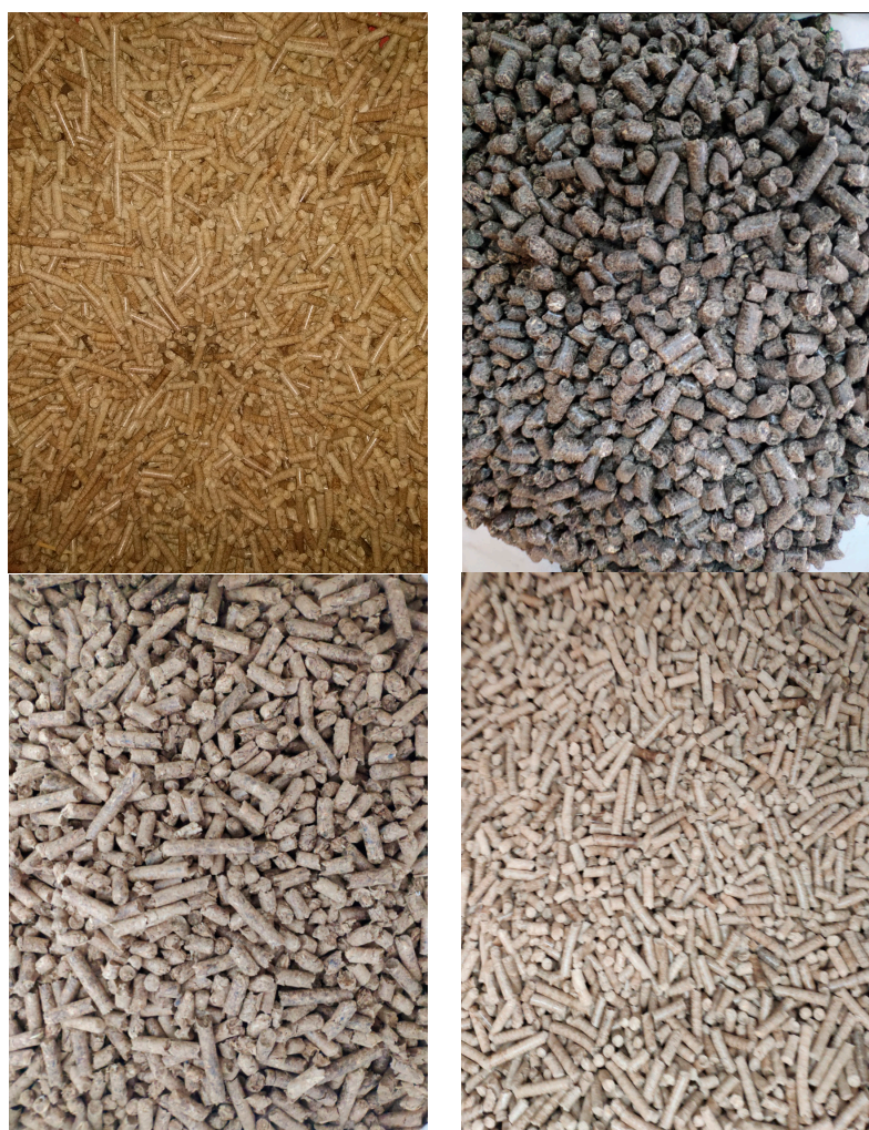
Figure 5. Experimental pellet pictures (wood pellet, (top left); sunflower husk pellet, (top right); miscanthus pellet, (bottom left); and corn stover pellet, (bottom right)).
