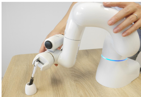
Fig. 1: Modeling the demonstrated trajectory through kinesthetic teaching is essential in imitation learning.
