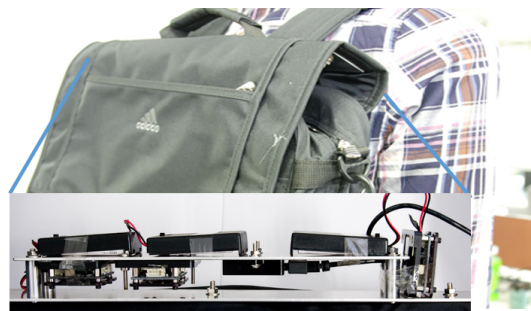
Figure 4. An example of three IMU sensors in the backpack for the test dataset. The sensors are attached to the top of the backpack.
