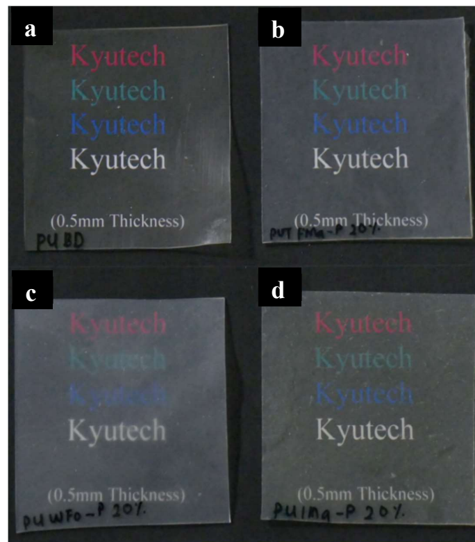
Figure 4.3: Images of PUs film after hot press; (a) PU BD (b) PU FMa-P 20% (c) PU WFo-P 20% (d) PU IMA-P 20%.
