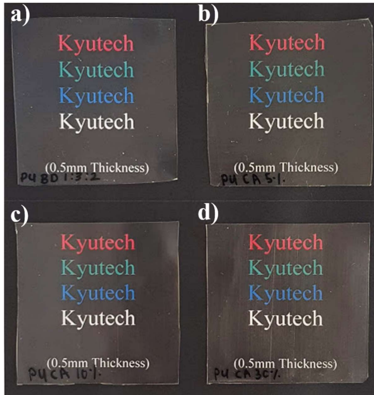
Figure 3.1: Morphological of (a) control PU BD and modified PUs with different weight percentage of cellulose acetate; (b) PU CA 5%, (c) PU CA 10%, and (d) PU CA 30%
