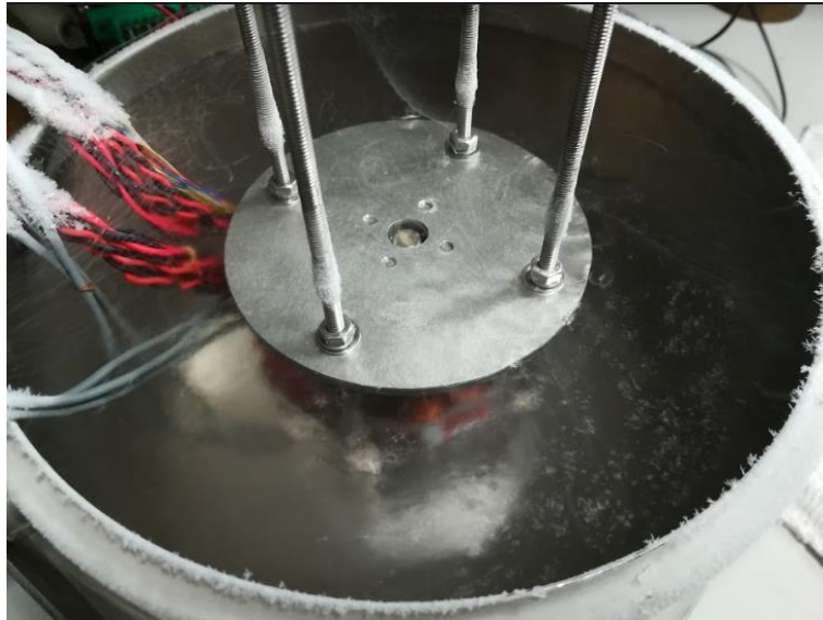
Fig. 2.16 Photograph of the experimental setup. The ASBM is set in liquid nitrogen. Levitation and rotation experiments are carried out using this setting.
