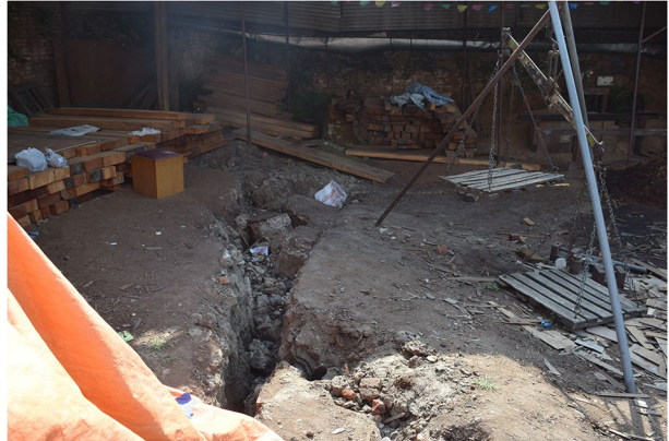
Fig. 4 Liquefaction and cracks in the ground at Kausaltar, Bhaktapur, Nepal, after the 2015 Gorkha earthquake, (Location 7a on Fig. 2). Photograph taken on 2015-05-31 [RM Pokhrel]
