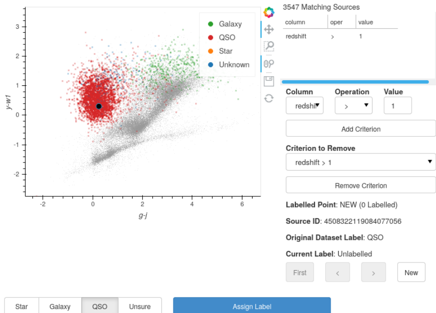
Figure 4: AstronomicAL enables the creation of curated test sets. The sample is selected according to user-defined criteria and verified visually. This test set can then be used during the active learning training process to ensure that the model will be sufficiently generalisable to future data.
