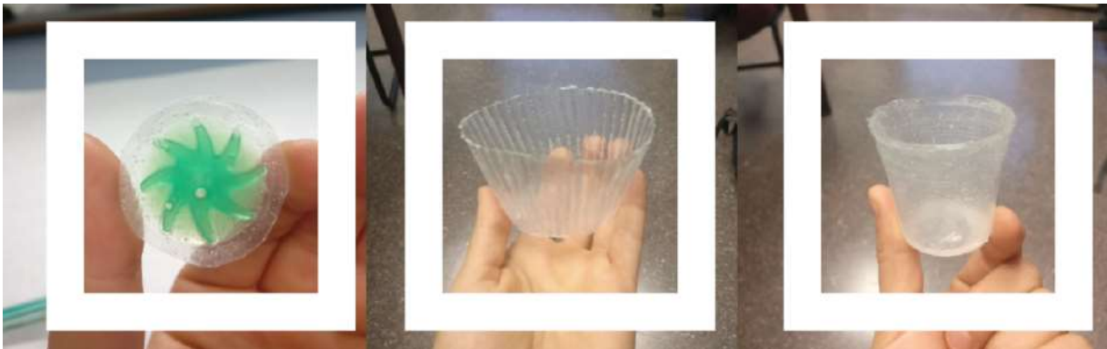
Figure B.2. Cellupack prototypes. Soluble packaging example made of HPC. From left to right: A single-dose toothpaste encapsulated in HPC, an ice-cream cup and an espresso coffee cup.
