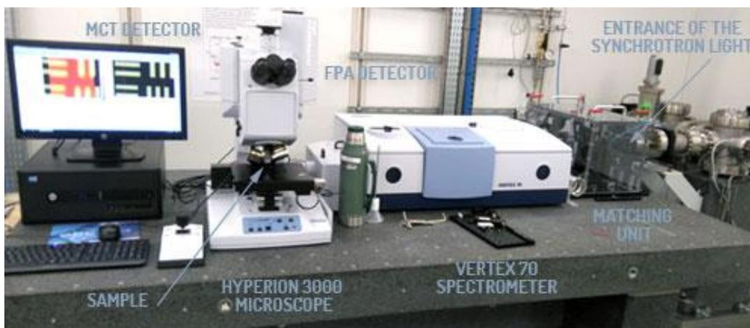
Figure 24. MIRAS beamline in ALBA Synchrotron (Source: <https://www.cells.es/en/beamlines/bl01-miras>)
