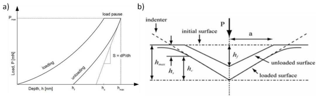
Figure 18. a) Typical load-displacement nanoindentation curve. b) Schematic illustration of the indenter and specimen surface at full load and unload and the parameters characterizing the contact geometry [98]
