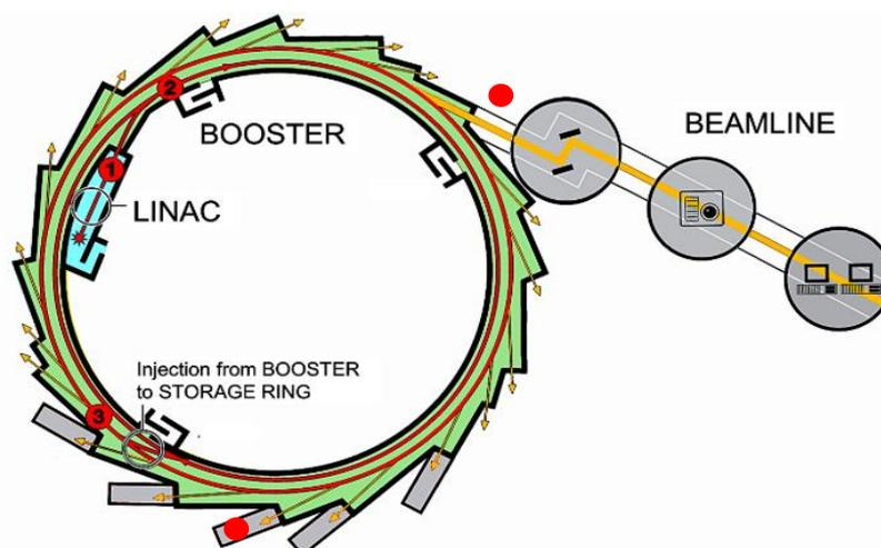
Figure 22. ALBA synchrotron scheme. 1. LINAC, 2. Booster ring, 3. Storage ring 4. Beamline [107]
