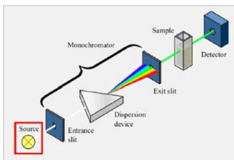
Figure 11. Spectrophotometer scheme
