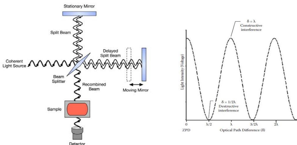
Figure 20. a. Michelson interferometer. b. Interferogram for a single wavelength of light passing through the interferometer (in real measurements, the interferogram obtained corresponds to many wavenumbers of light passing through the interferometer together).
