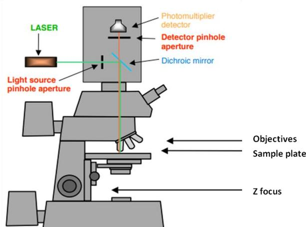
Figure 16. Confocal microscope scheme
