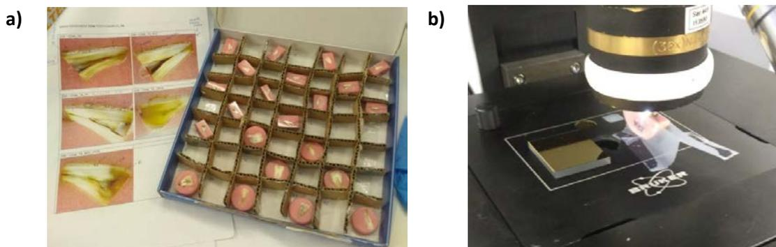
Figure 21. a) Tooth samples with specular polishing. b) FTIR microscope objective pointing on the sample; at its side, a golden mirror (perfect mirror) used as a reference to acquire the reflectance baseline.
