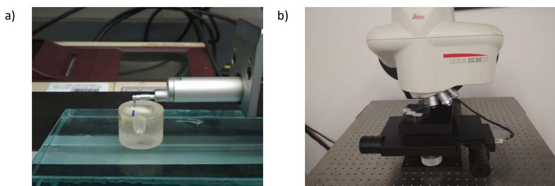
Figure 19.a. Stylus profilometer. b. Optical profilometer
