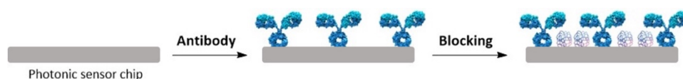
Figure 3.12. Scheme of the physical adsorption of the antibody and the blocking step.
